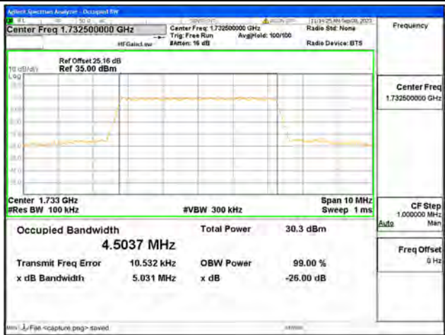
B4 / 5MHz / 16QAM/ Mid CH
