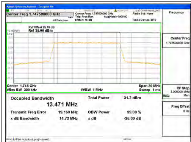
B4 / 15MHz / QPSK/ High CH
