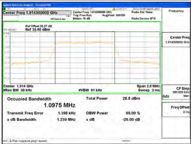
B25 / 1.4MHz / 64QAM/ High CH
