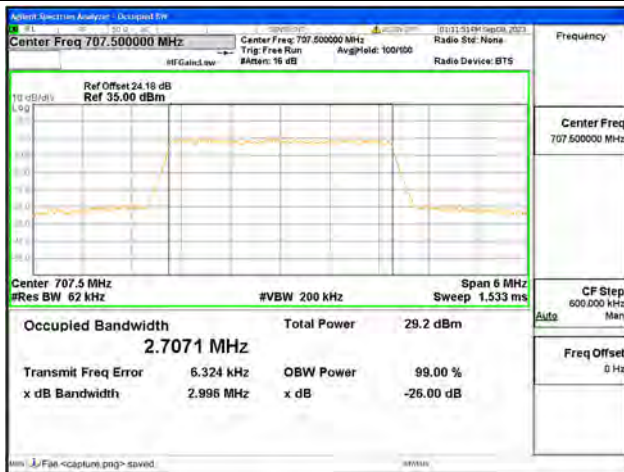
B12 / 3MHz / 64QAM/ Mid CH
