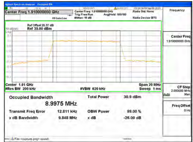
B25 / 10MHz / QPSK/ High CH
