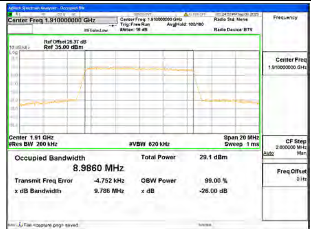
B25 / 10MHz / 64QAM/ High CH
