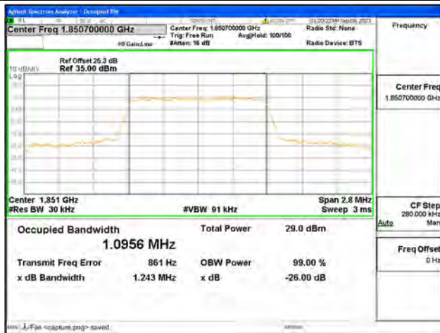
B25 / 1.4MHz / 64QAM/ Low CH
