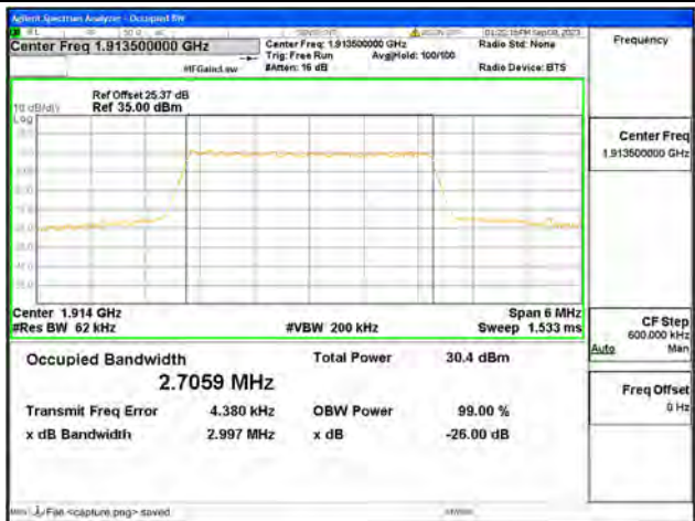
B25 / 3MHz / 16QAM/ High CH
