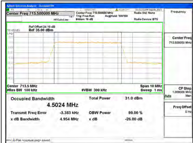
B12 / 5MHz / QPSK/ High CH
