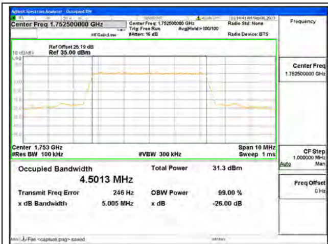
B4 / 5MHz / QPSK/ High CH
