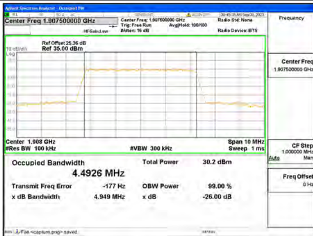
B2 / 5MHz / 64QAM/ High CH
