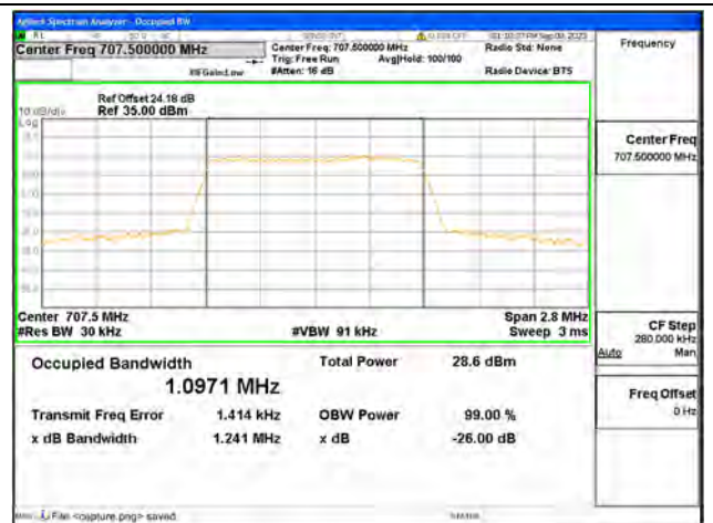
B12 / 1.4MHz / 64QAM/ Mid CH
