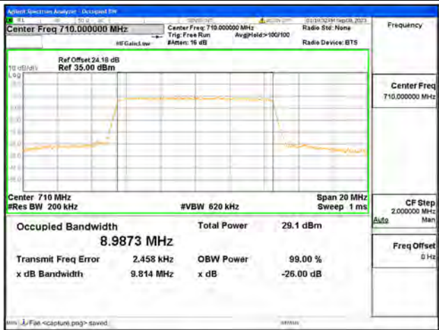
B17 / 10MHz / 64QAM/ Mid CH
