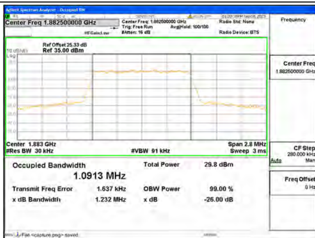
B25 / 1.4MHz / 16QAM/ Mid CH
