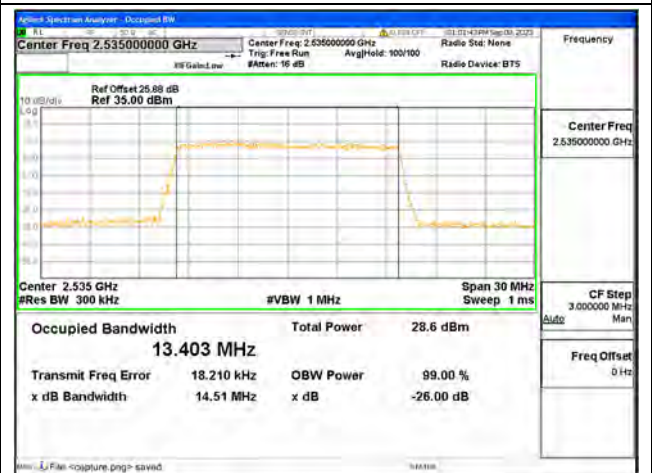
B7 / 15MHz / 64QAM/ Mid CH
