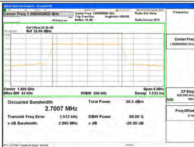
B2 / 3MHz / 16QAM/ High CH
