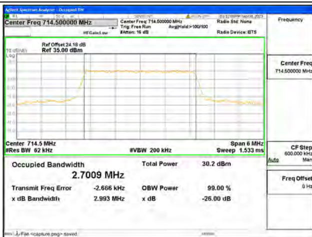
B12 / 3MHz / 16QAM/ High CH
