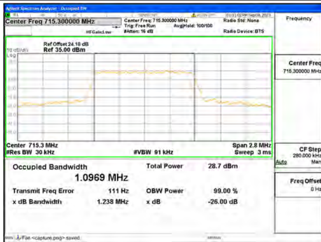
B12 / 1.4MHz / 64QAM/ High CH
