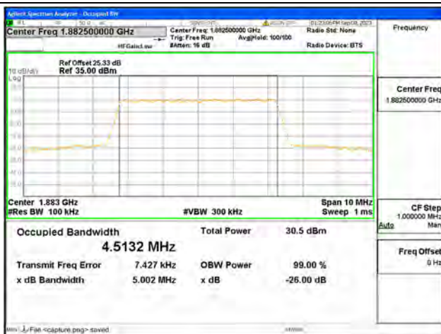
B25 / 5MHz / 16QAM/ Mid CH
