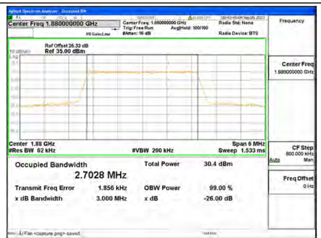
B2 / 3MHz / 16QAM/ Mid CH
