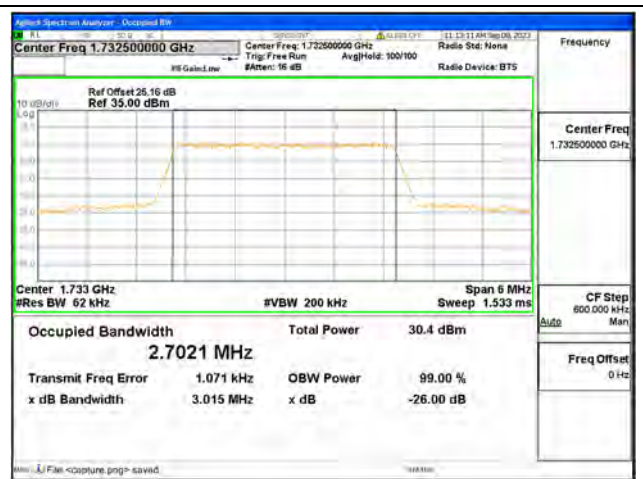
B4 / 3MHz / 16QAM/ Mid CH
