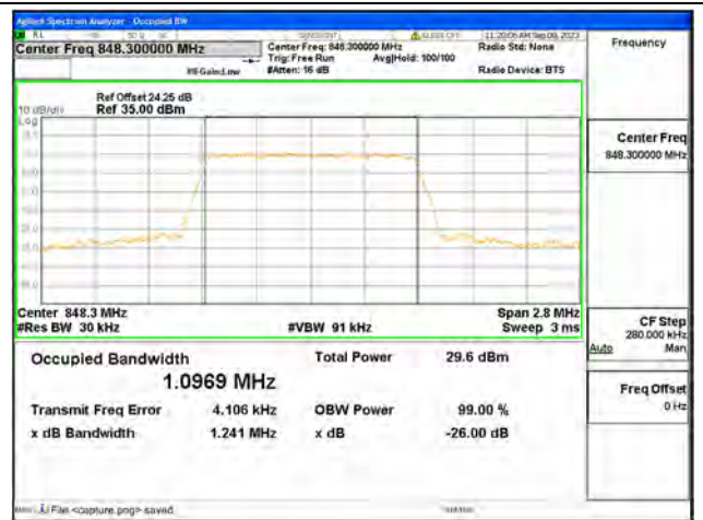
B5 / 1.4MHz / 16QAM/ High CH
