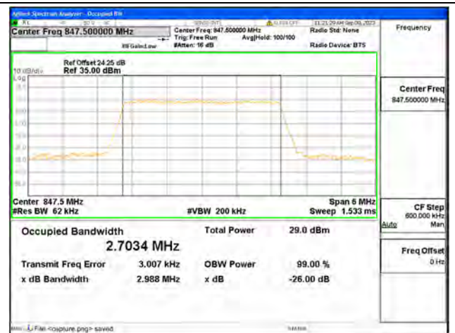
B5 / 3MHz / 64QAM / High CH
