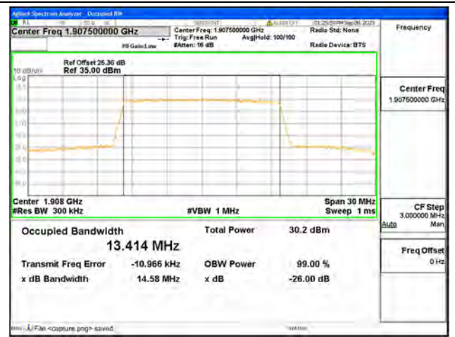
B25 / 15MHz / 16QAM/ High CH
