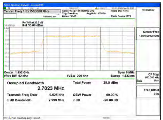
B25 / 3MHz / 64QAM/ Low CH
