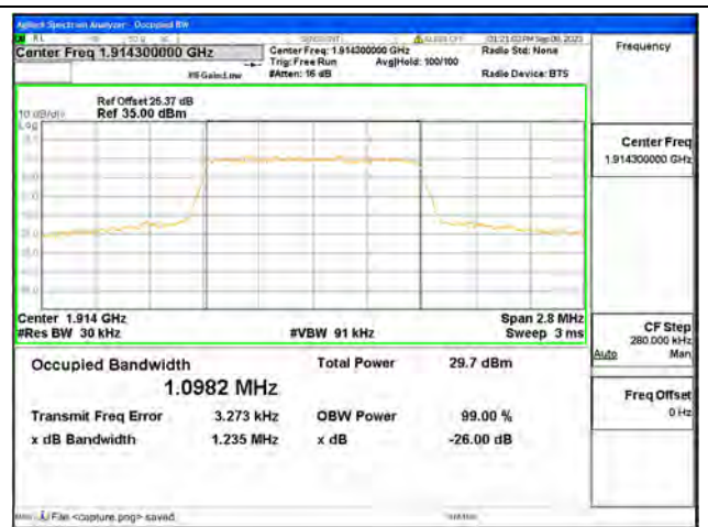
B25 / 1.4MHz / 16QAM/ High CH
