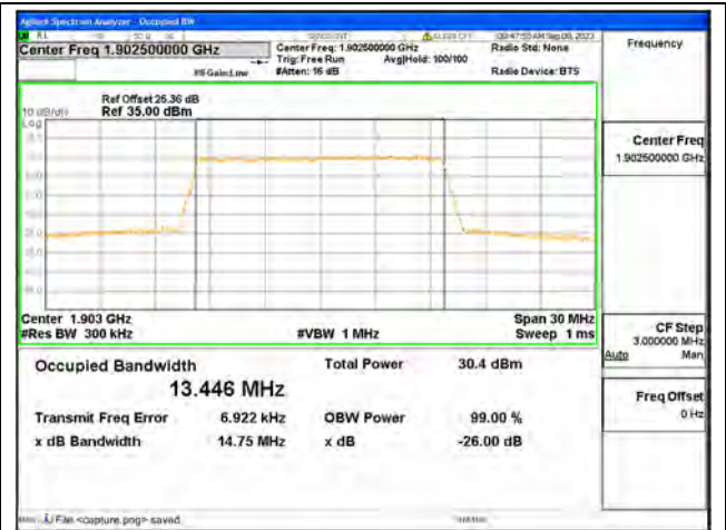
B2 / 15MHz / 16QAM/ High CH
