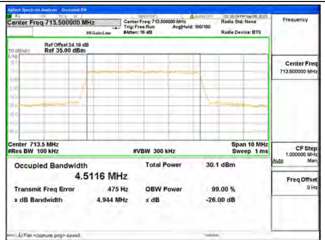
B17 / 5MHz / 16QAM/ High CH
