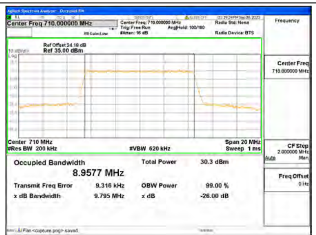
B17 / 10MHz / 16QAM/ Mid CH
