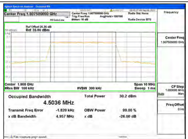
B2 / 5MHz / 16QAM/ High CH
