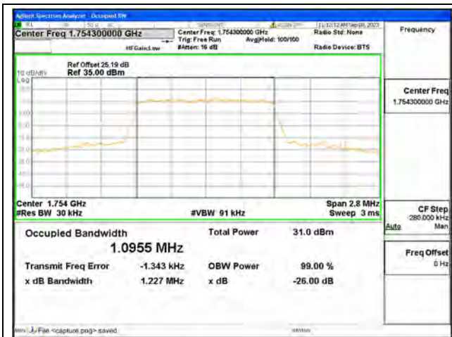
B4 / 1.4MHz / QPSK/ High CH
