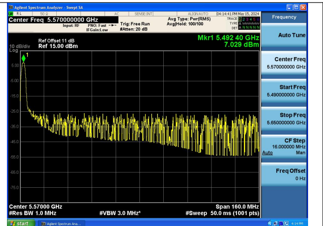
Mode:802.11ax HE160 Tone:26T Frequency:5570MHz Ant:Chain1
