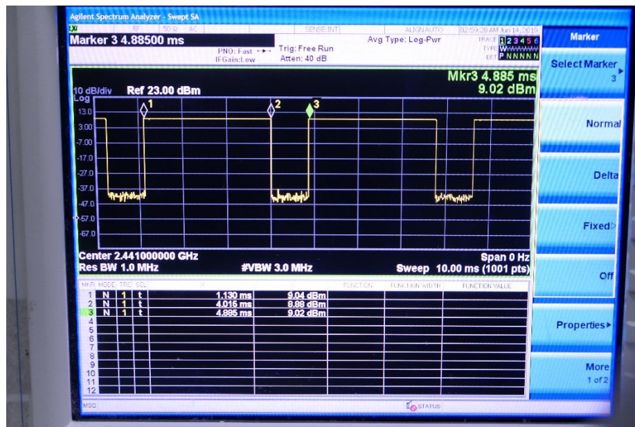
Time-domain plot for Bluetooth transmission signal
