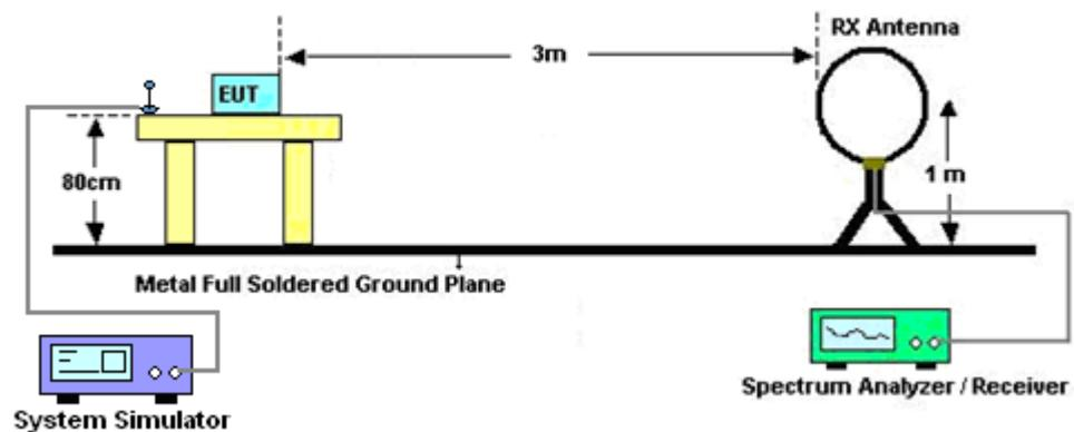
For radiated test from 30MHz to 1GHz
