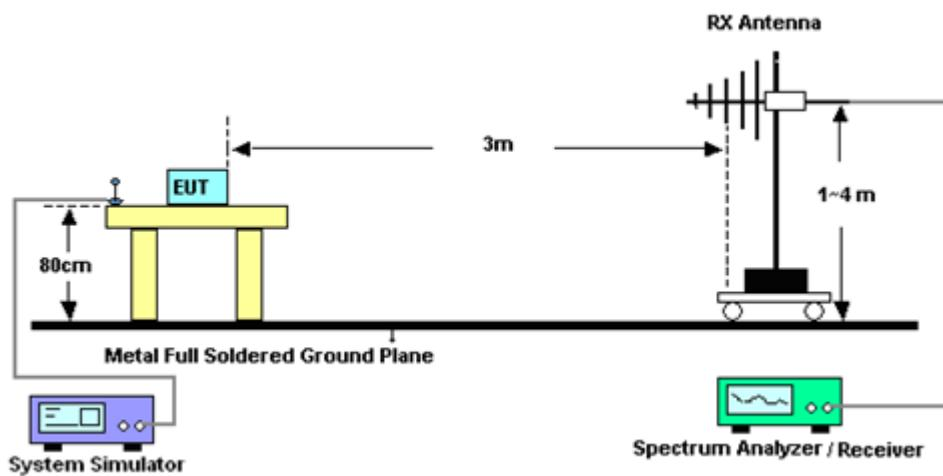
For radiated test from 1GHz to 18GHz
