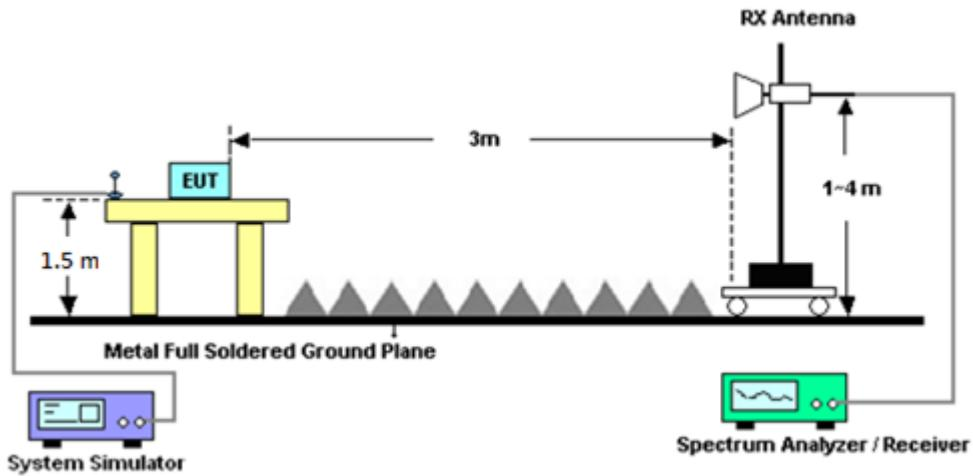
For radiated test above 18GHz
