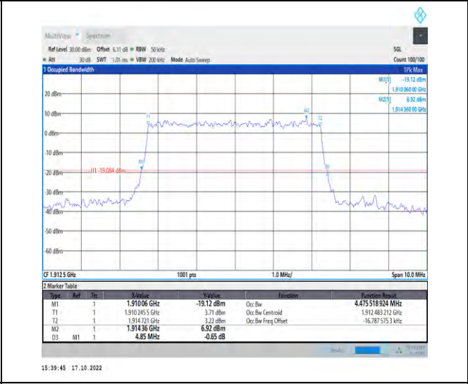
1-N25-PC3-15-5-H-9-CP-256QAM-Outer_Full-25@0-A Ant1-4.476-4.850- \leq 5-PASS
