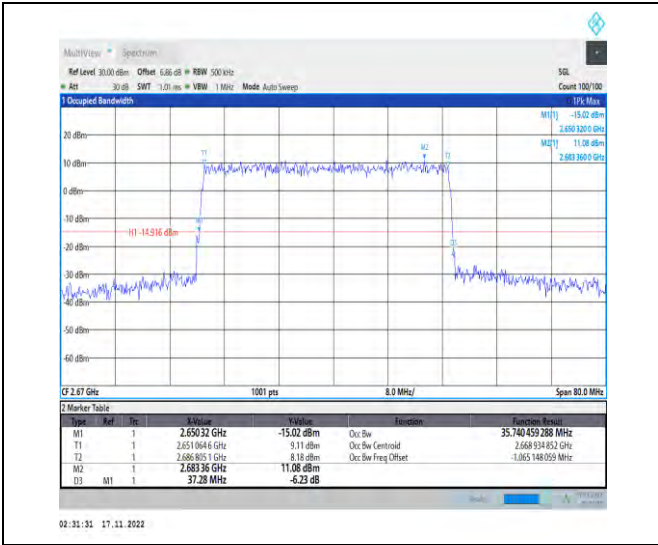
1-N41-PC2-30-40-H-3-DFT-16QAM-Outer_Full-100 @0-Ant1-35.74-37.280-≤40-PASS
