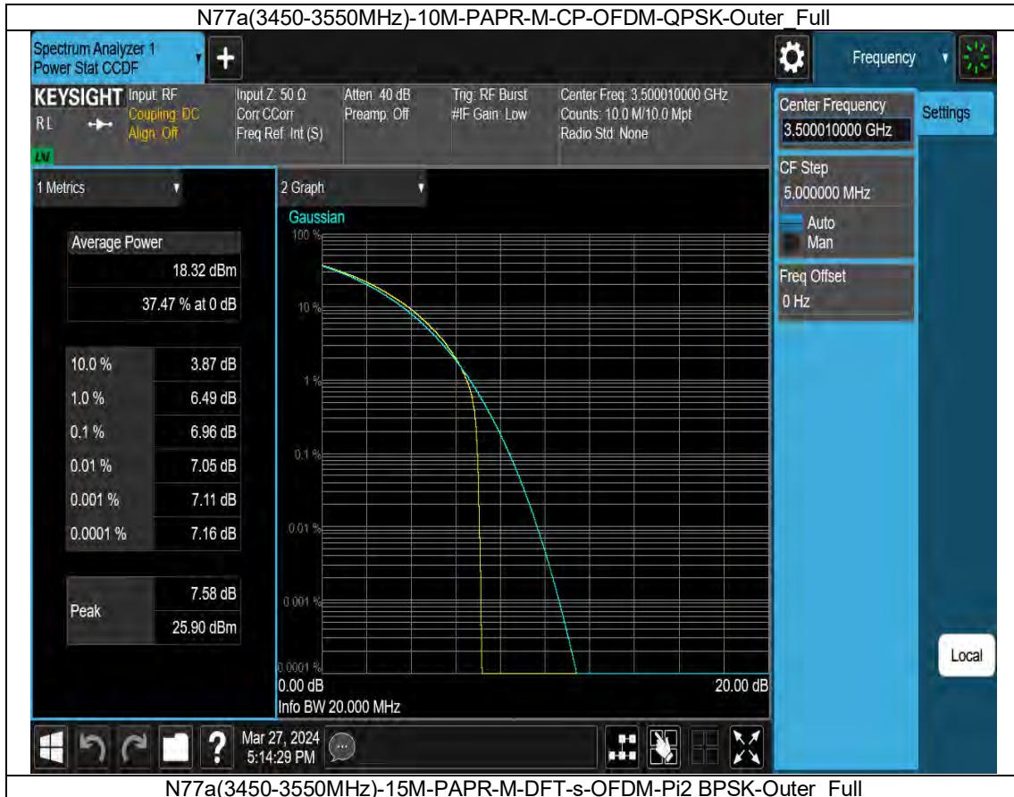
N77a(3450-3550MHz)-15M-PAPR-M-DFT-s-OFDM-Pi2 BPSK-Outer Full
