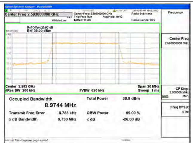
Band41 / 10MHz / 16QAM/ Mid CH
