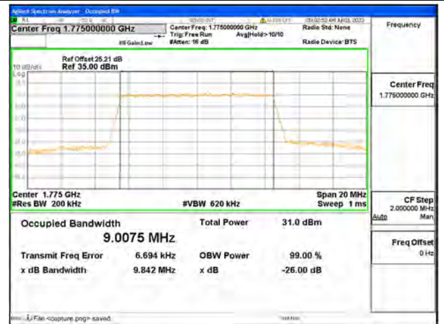
Band66 / 10MHz / QPSK/ High CH
