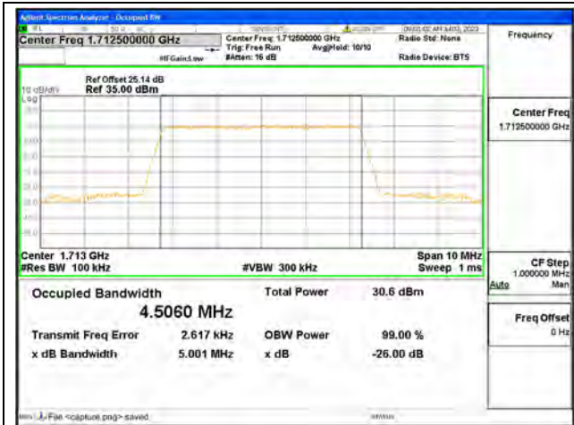
Band66 / 5MHz / QPSK/ Low CH
