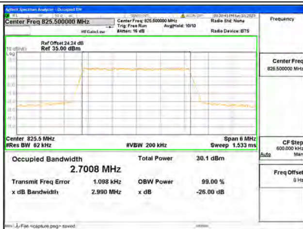
Band26 Part22 / 3MHz / 16QAM/ Low CH
