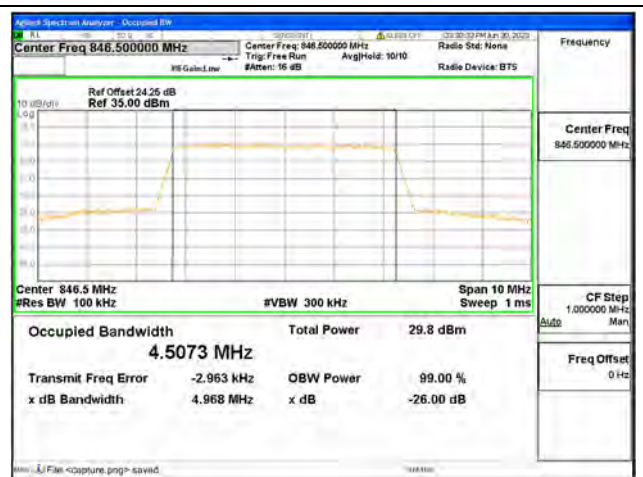
Band26 Part22 / 5MHz / 16QAM/ High CH
