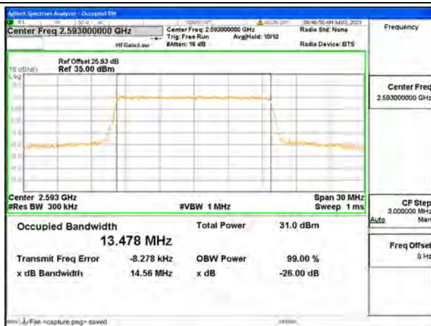
Band41 / 15MHz / 16QAM/ Mid CH
