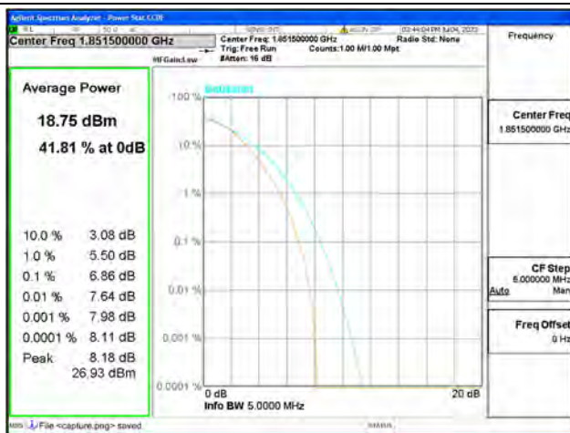
Band2 / 3MHz / Low CH / 16QAM
