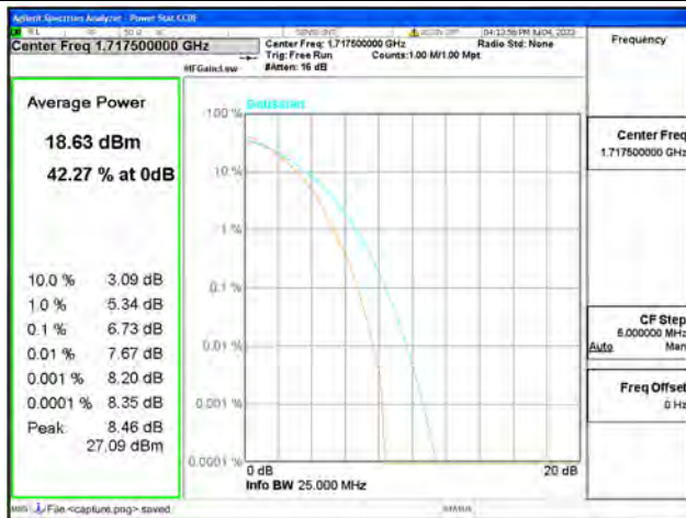
Band4 / 15MHz / Low CH / 64QAM
