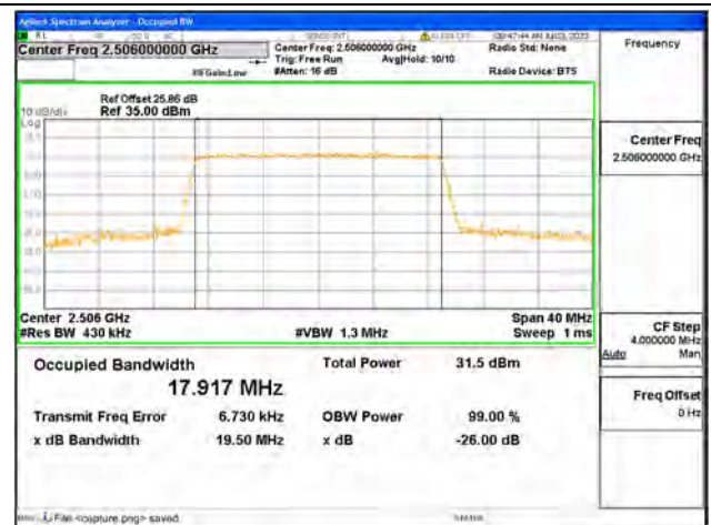
Band41 / 20MHz / 64QAM/ Low CH
