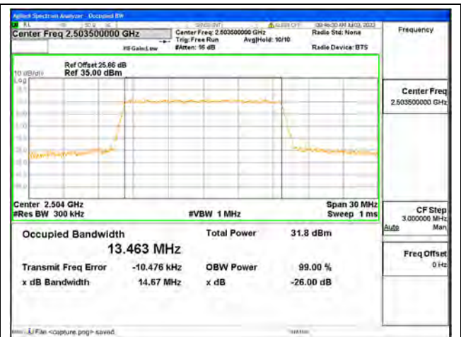
Band41 / 15MHz / 16QAM/ Low CH
