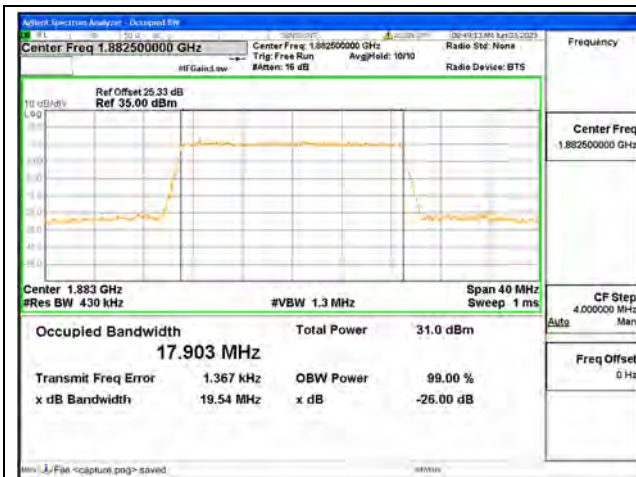
Band25 / 20MHz / QPSK/ Mid CH
