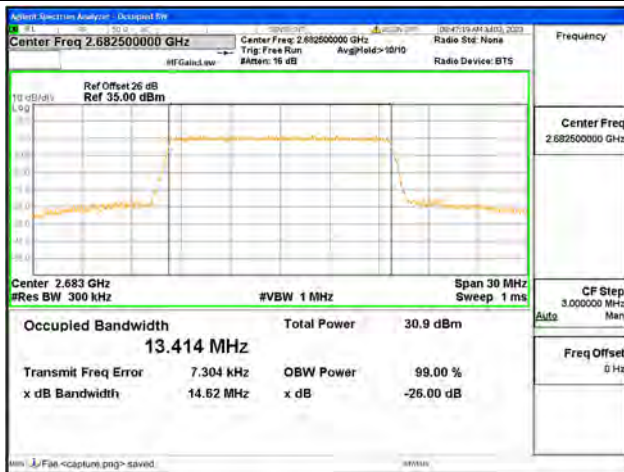
Band41 / 15MHz / 64QAM/ High CH
