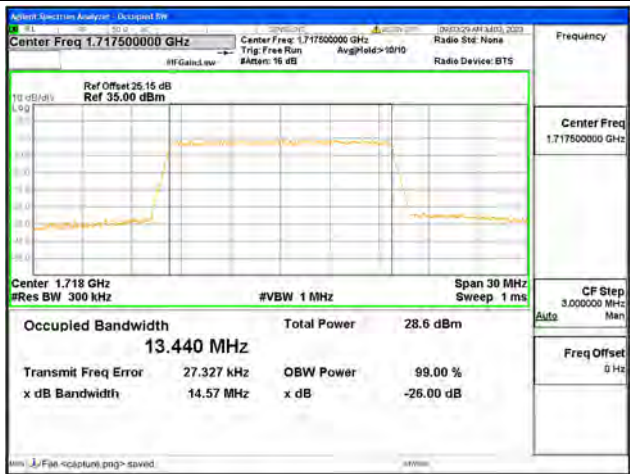
Band66 / 15MHz / 64QAM/ Low CH
