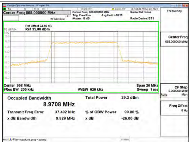
Band71 / 10MHz / 16QAM/ Low CH
