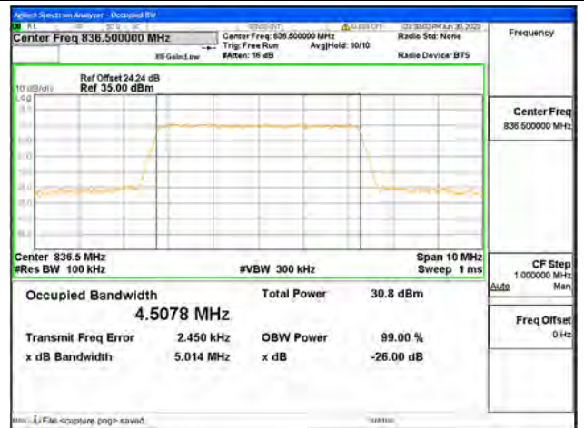
Band26 Part22 / 5MHz / QPSK/ Mid CH
