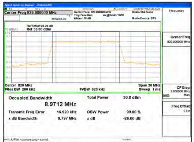
Band26 Part22 / 10MHz / QPSK/ Low CH
