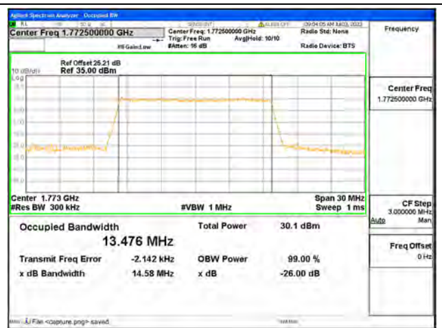
Band66 / 15MHz / 16QAM/ High CH
