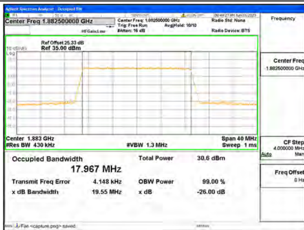
Band25 / 20MHz / 64QAM/ Mid CH
