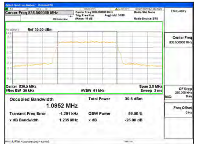
Band26 Part22 / 1.4MHz / QPSK/ Mid CH
