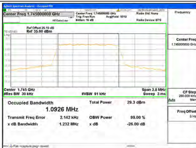
Band66 / 1.4MHz / 16QAM/ Mid CH
