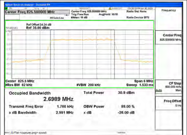
Band26 Part22 / 3MHz / QPSK/ Low CH
