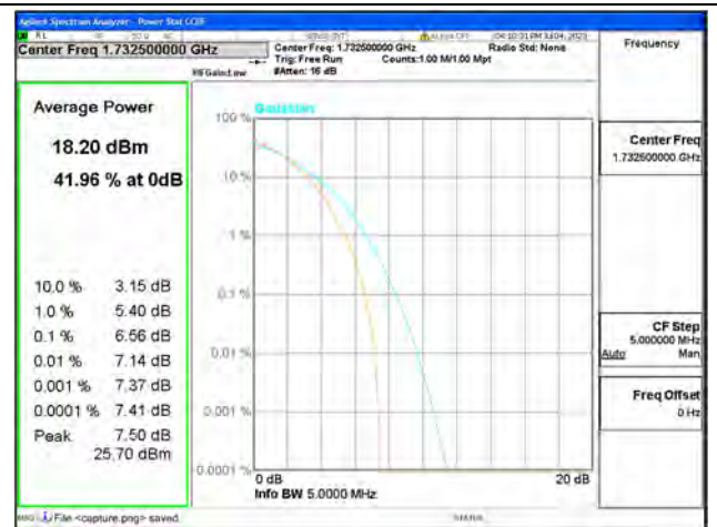
Band4 / 1.4MHz / Mid CH / 64QAM
