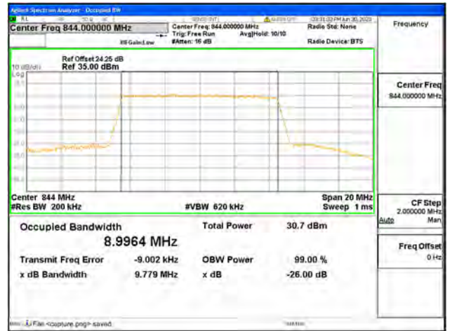
Band26 Part22 / 10MHz / QPSK/ High CH
