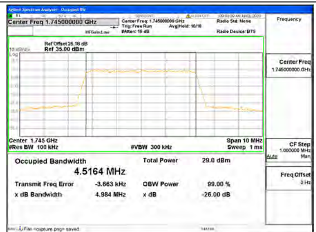
Band66 / 5MHz / 64QAM/ Mid CH
