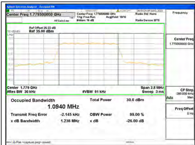
Band66 / 1.4MHz / QPSK/ High CH
