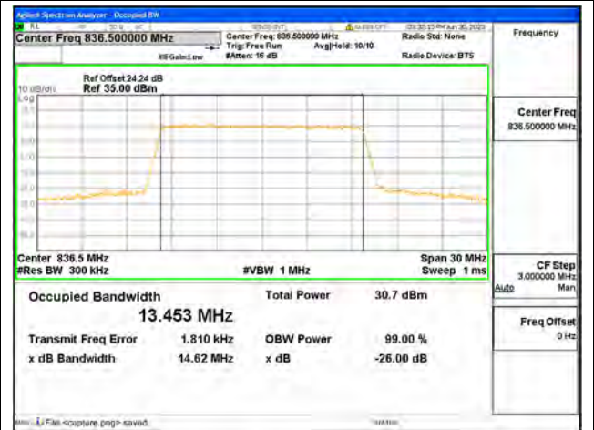
Band26 Part22 / 15MHz / QPSK/ Mid CH
