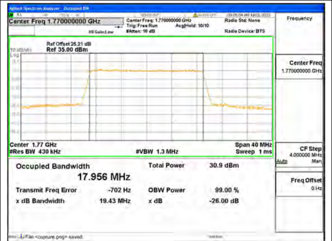
Band66 / 20MHz / QPSK/ High CH
