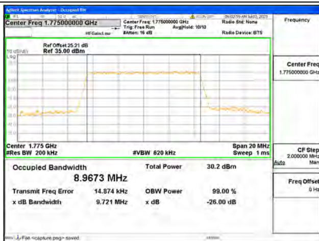
Band66 / 10MHz / 16QAM/ High CH
