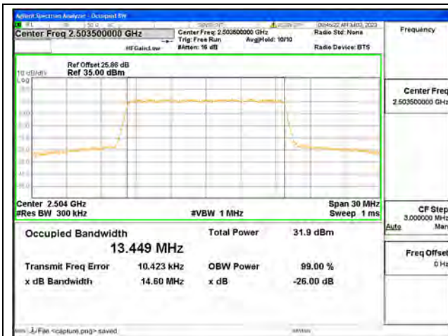
Band41 / 15MHz / QPSK/ Low CH
