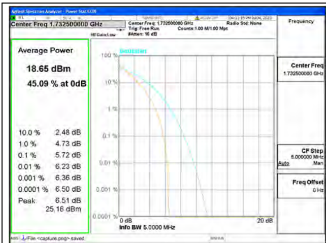
Band4 / 3MHz / Mid CH / QPSK
