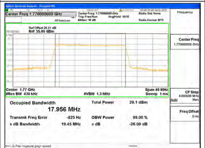
Band66 / 20MHz / 64QAM/ High CH
