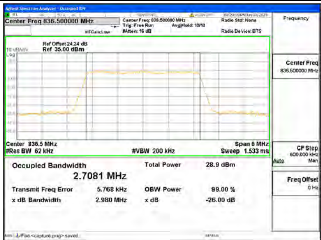
Band26 Part22 / 3MHz / 64QAM/ Mid CH
