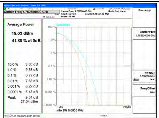
Band4 / 5MHz / High CH / 16QAM
