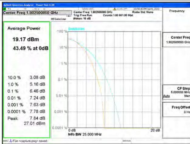
Band2 / 15MHz / High CH / 64QAM
