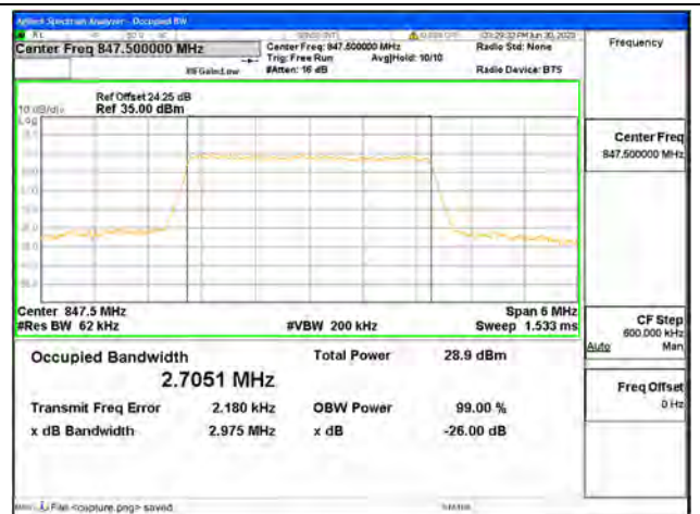
Band26 Part22 / 3MHz / 64QAM/ High CH
