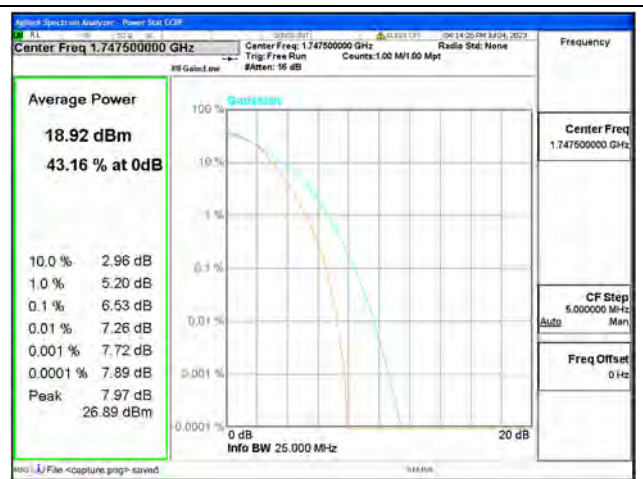
Band4 / 15MHz / High CH / 16QAM
