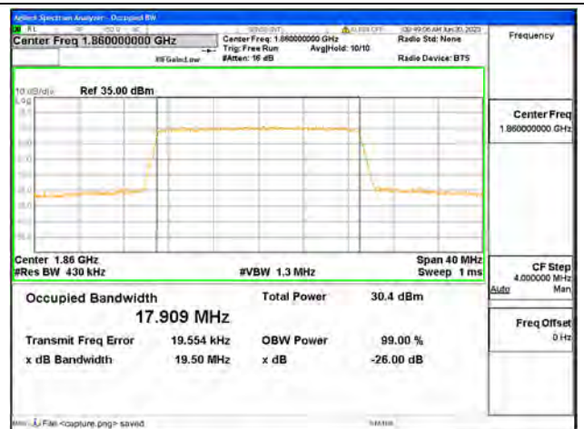
Band25 / 20MHz / 64QAM/ Low CH
