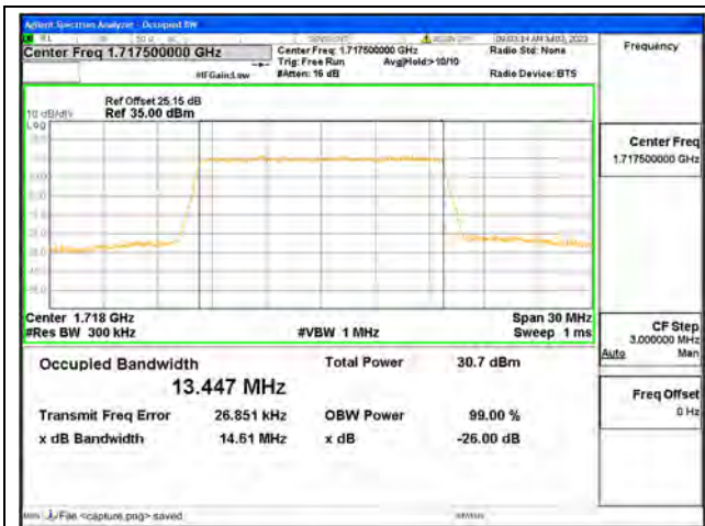
Band66 / 15MHz / QPSK/ Low CH
