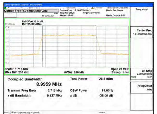
Band66 / 10MHz / 64QAM/ Low CH
