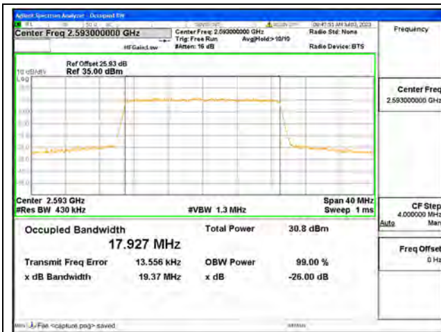
Band41 / 20MHz / QPSK/ Mid CH
