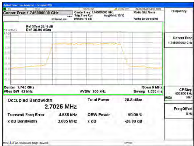
Band66 / 3MHz / 64QAM/ Mid CH
