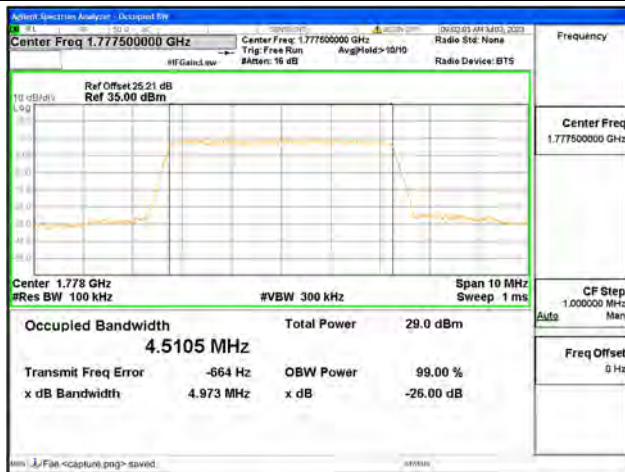
Band66 / 5MHz / 64QAM/ High CH
