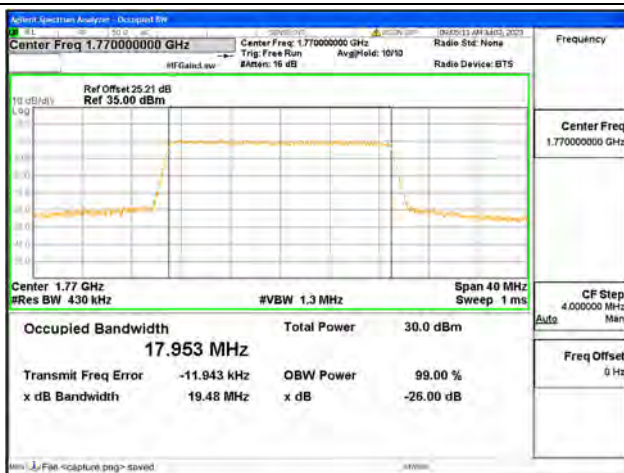
Band66 / 20MHz / 16QAM/ High CH
