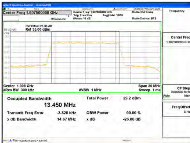
Band25 / 15MHz / 64QAM/ High CH
