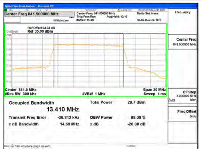
Band26 Part22 / 15MHz / 16QAM/ High CH
