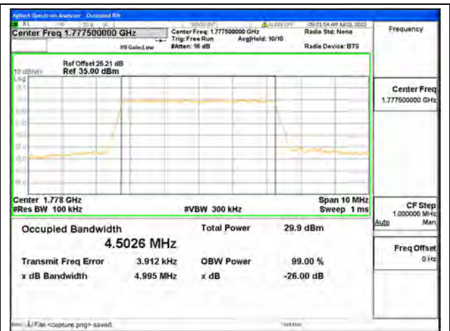
Band66 / 5MHz / 16QAM/ High CH
