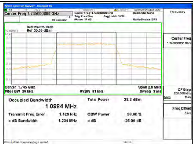
Band66 / 1.4MHz / 64QAM/ Mid CH
