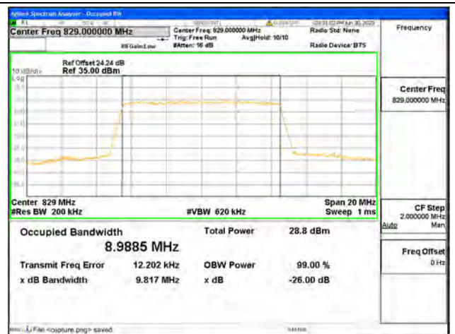
Band26 Part22 / 10MHz / 64QAM/ Low CH
