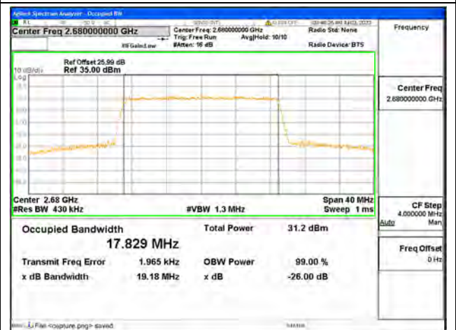
Band41 / 20MHz / 64QAM/ High CH
