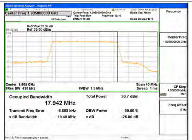
Band25 / 20MHz / 64QAM/ High CH
