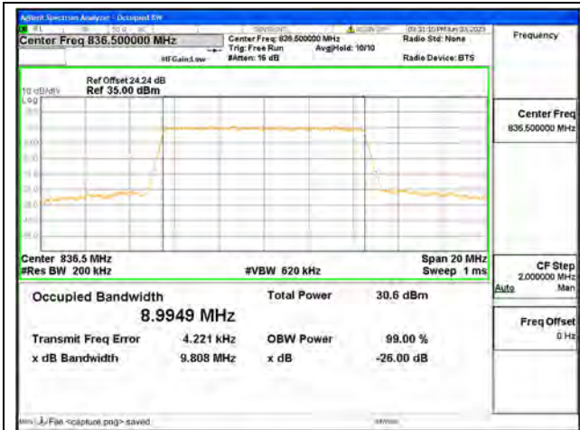
Band26 Part22 / 10MHz / QPSK/ Mid CH
