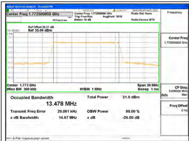
Band66 / 15MHz / QPSK/ High CH
