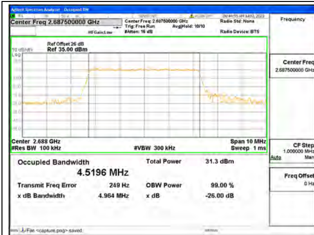
Band41 / 5MHz / QPSK/ High CH
