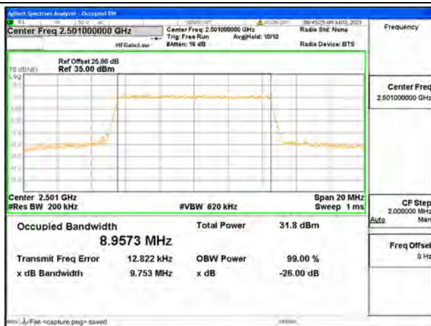
Band41 / 10MHz / 16QAM/ Low CH
