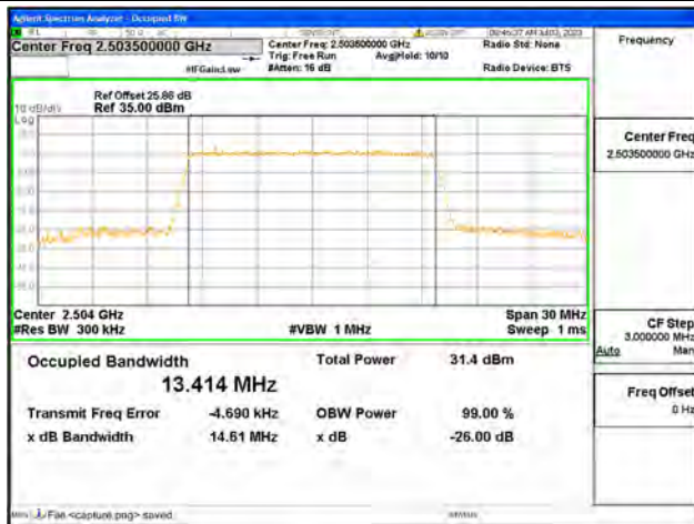
Band41 / 15MHz / 64QAM/ Low CH
