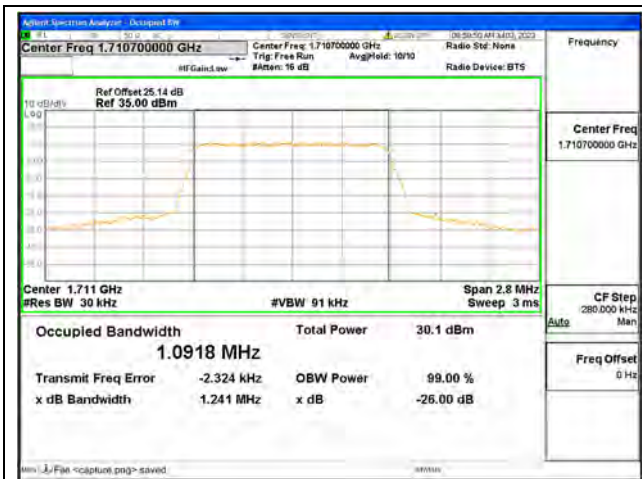
Band66 / 1.4MHz / QPSK/ Low CH
