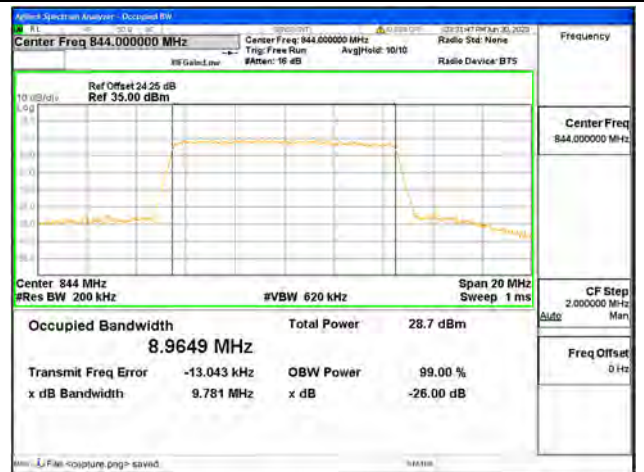
Band26 Part22 / 10MHz / 64QAM/ High CH
