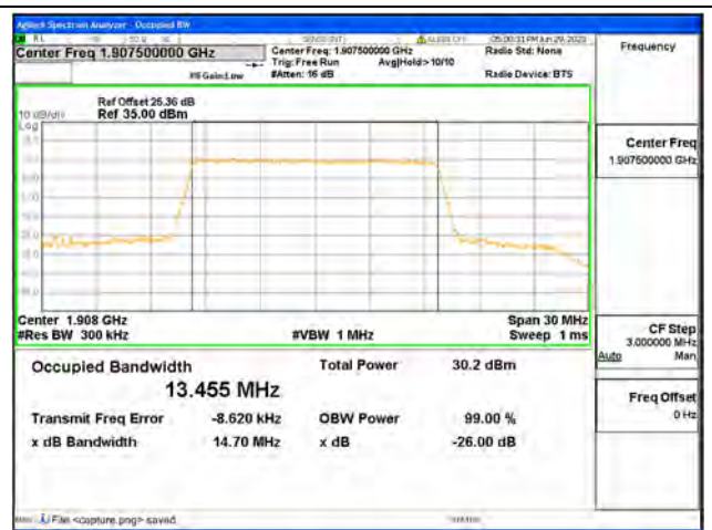
Band25 / 15MHz / 16QAM/ High CH
