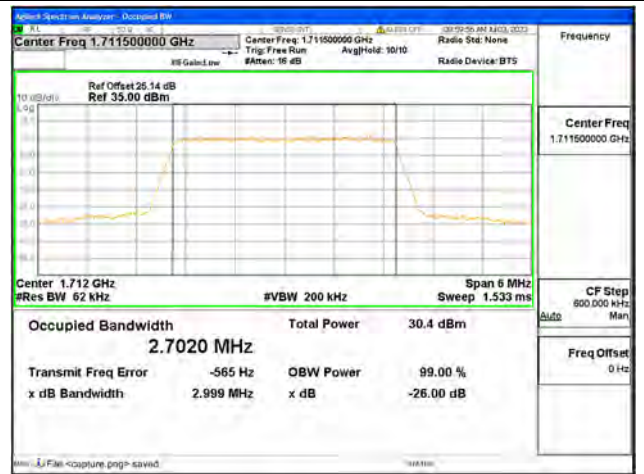
Band66 / 3MHz / QPSK/ Low CH
