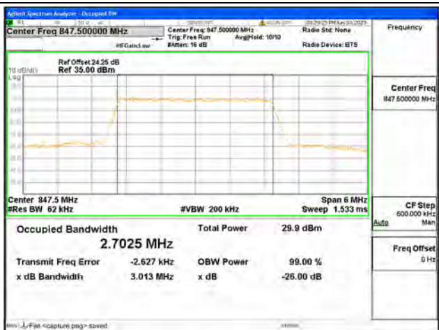
Band26 Part22 / 3MHz / 16QAM/ High CH
