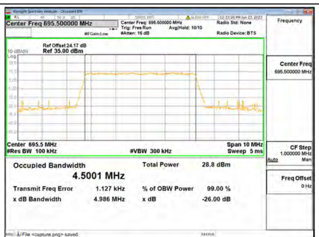
Band71 / 5MHz / 16QAM/ High CH
