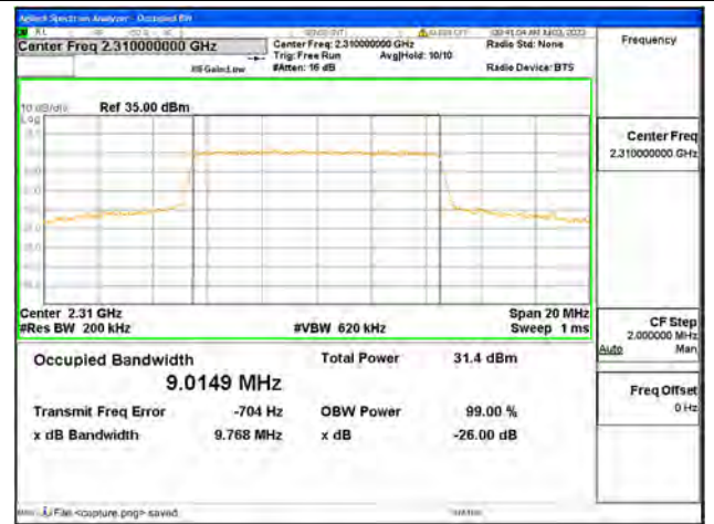
Band30 / 10MHz / QPSK/ Mid CH
