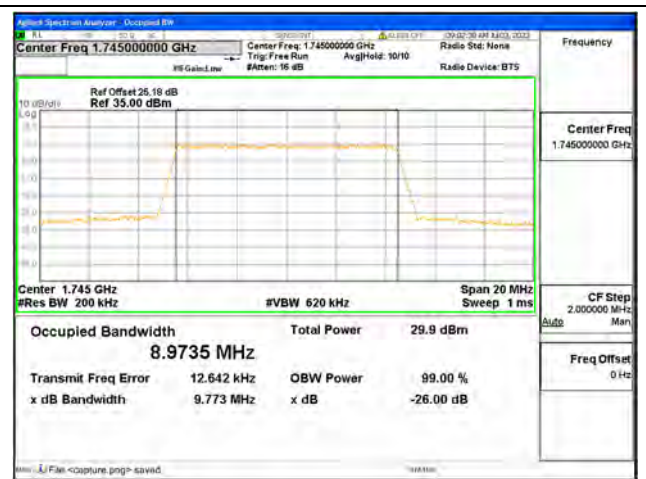
Band66 / 10MHz / 16QAM/ Mid CH
