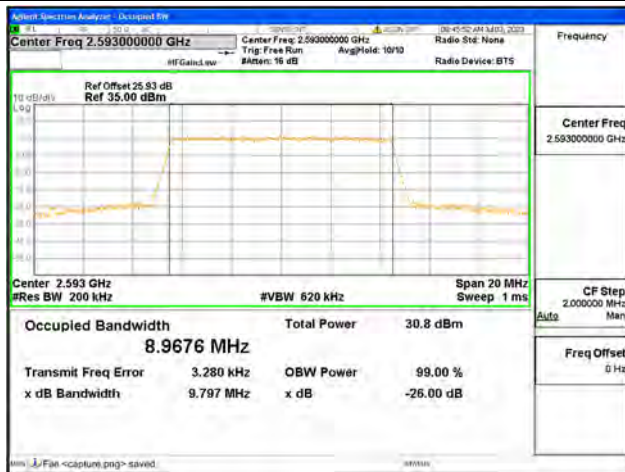
Band41 / 10MHz / 64QAM/ Mid CH
