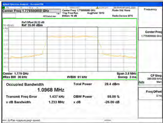
Band66 / 1.4MHz / 64QAM/ High CH
