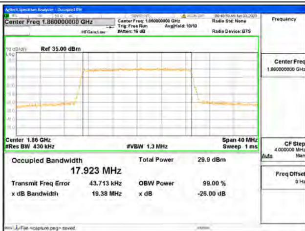
Band25 / 20MHz / 16QAM/ Low CH
