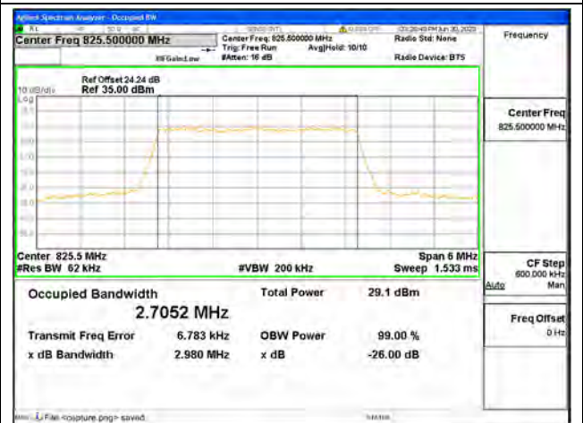
Band26 Part22 / 3MHz / 64QAM/ Low CH
