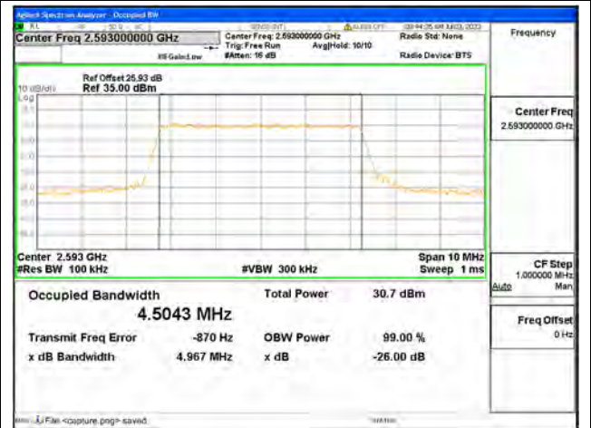
Band41 / 5MHz / QPSK/ Mid CH
