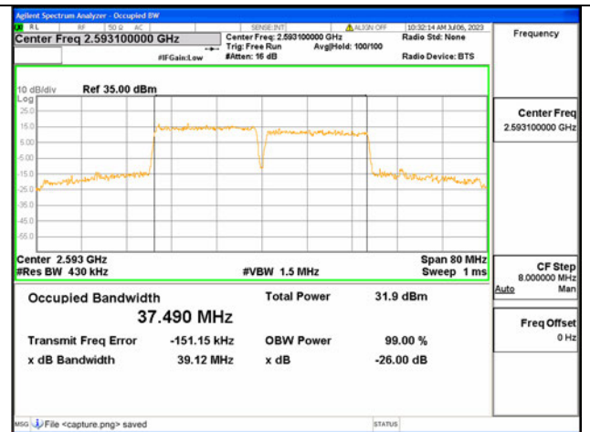
41C / 20+20MHz / 64QAM/ Mid CH
