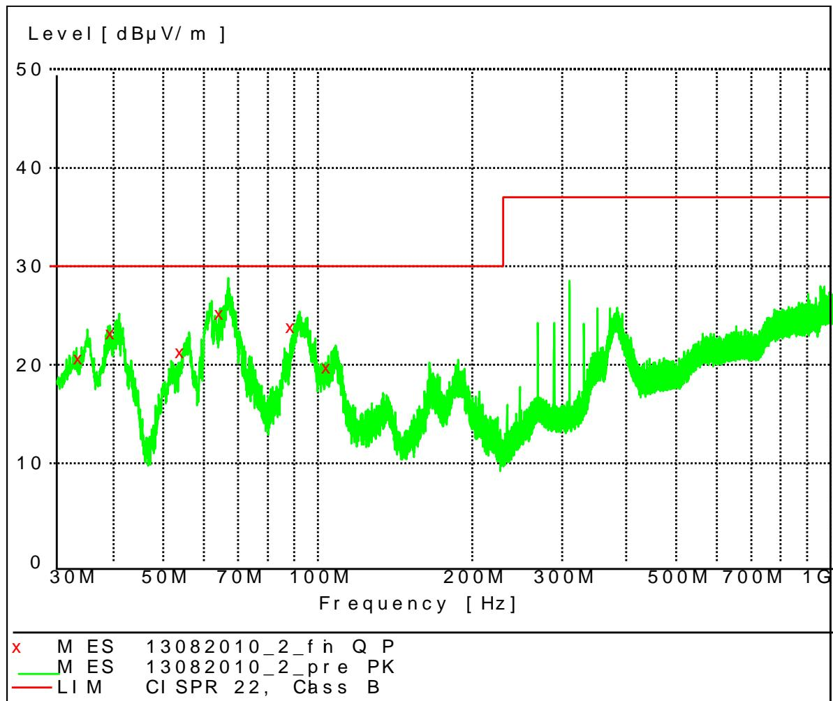
Horizontal and vertical polarizations in the frequency range 30 - 1000 MHz measured by using the peak detector. During the peak detector scan, the turntable was rotated from 0° to 360° with 30° steps with the antenna heights 1.0 m and 3.0 m. The highest levels of the radiated interference field strength measured by using the quasi-peak detector were recorded.
