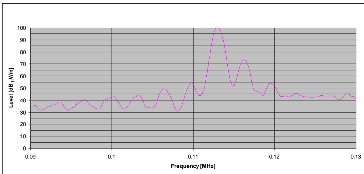
90 kHz – 110 kHz restricted band measured with the peak detector at 3 m measuring distance.
