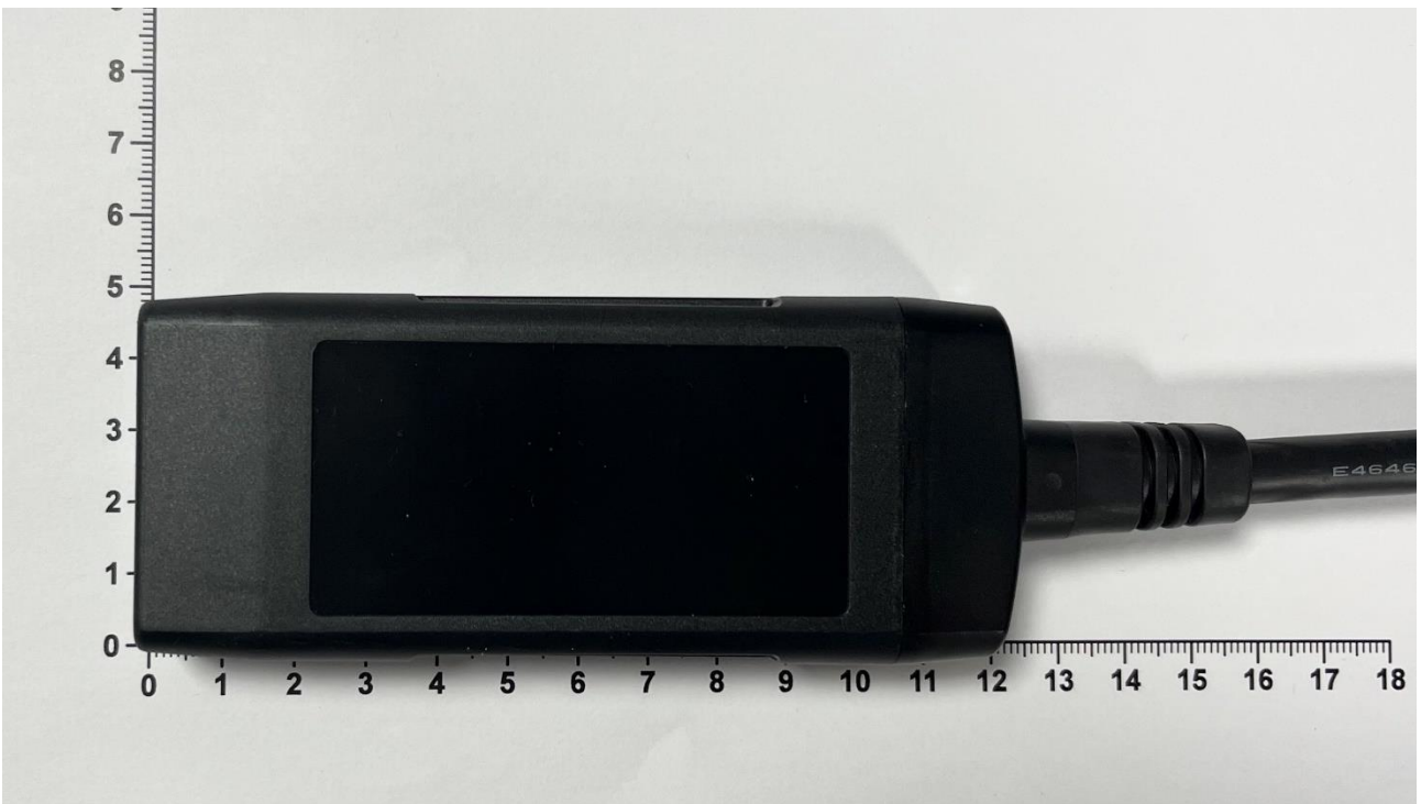
TU700-5 without the back label and the mounting cradle seen from the back
