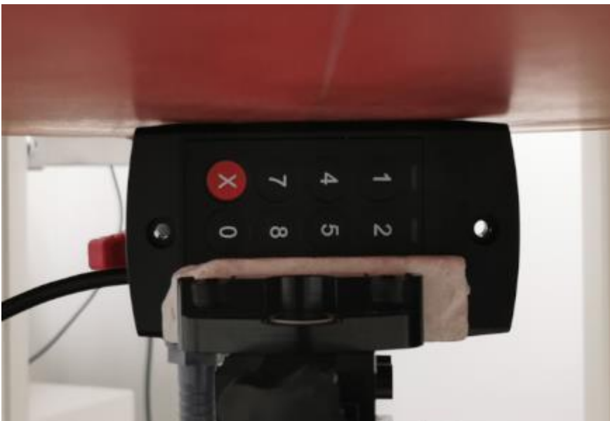
Figure 6 The left of the DUT against the phantom with 0mm separation
