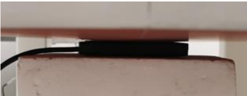
Figure 4 The front of the DUT against the phantom with 0mm separation
