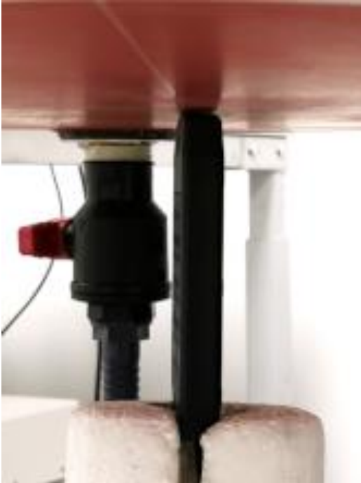
Figure 7 The top of the DUT against the phantom with 0mm separation
