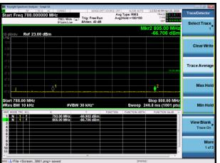
NB-IOT Band 13 QPSK 15kHz (763MHz ~775MHz)
