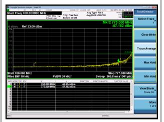
NB-IOT Band 13 BPSK 3.75kHz (793MHz ~805MHz)
