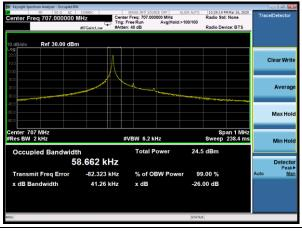
NB-IOT Band 71 QPSK 15kHz 12@0 CH-High
