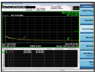
NB-IOT Band 13 QPSK 3.75kHz (763MHz ~775MHz)
