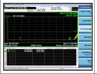
NB-IOT Band 13 BPSK 15kHz (793MHz ~805MHz)
