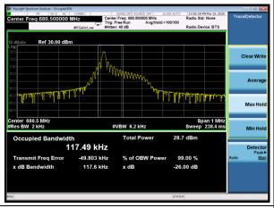
NB-IOT Band 71 QPSK 3.75kHz 1@0 CH-High
