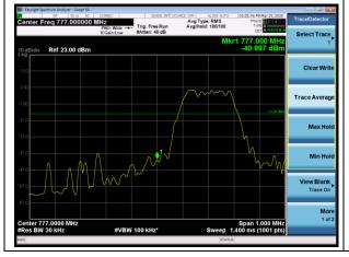
NB-IOT Band 13 QPSK 15kHz 12@0 CH-High
