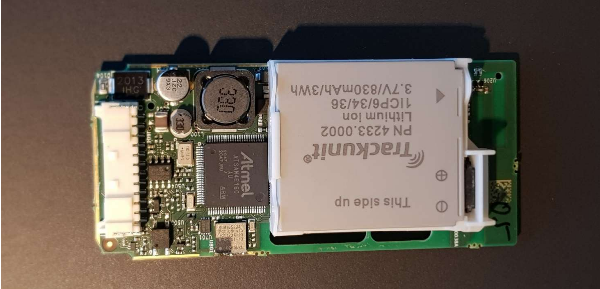
TU600A Print seen from the top with battery model 1-830mAh (Actec)
