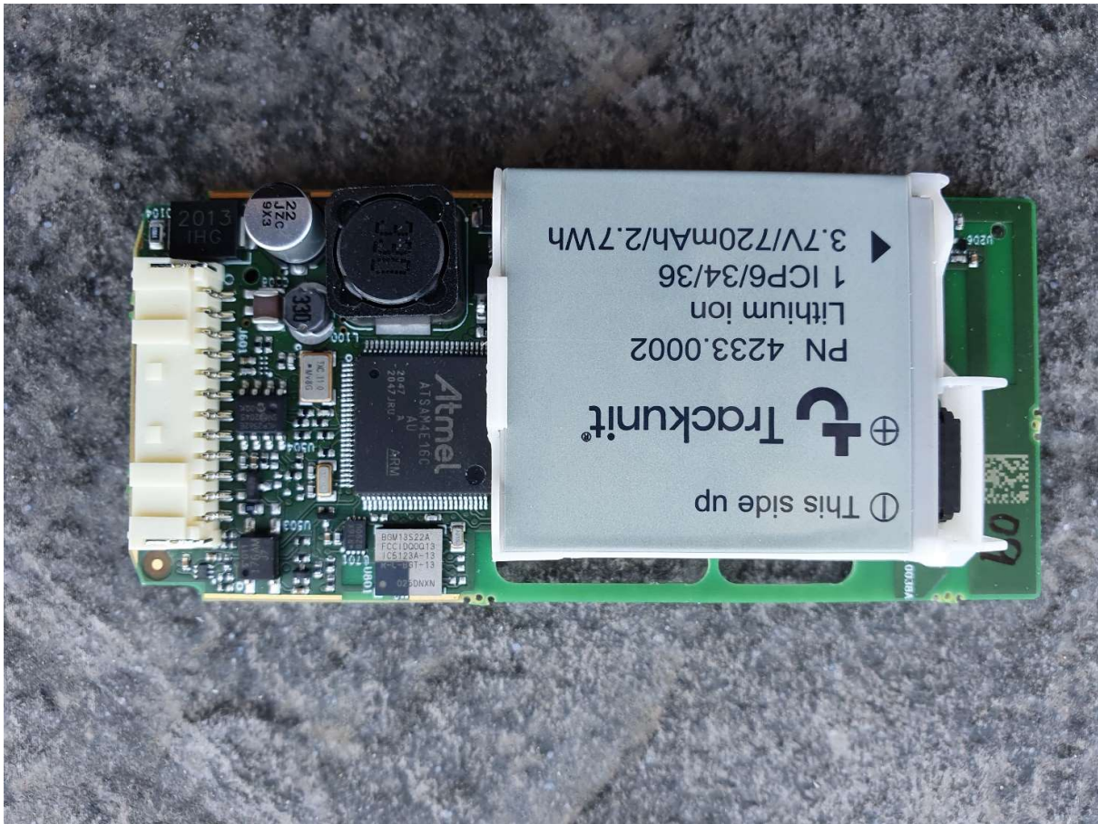
TU600A Print seen from the top with battery model 2-720 mAh (Duracell)
