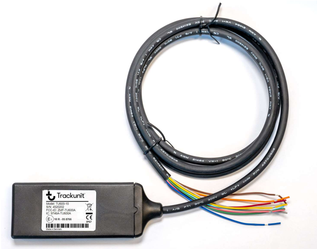
TU600-15 seen from the back with its power/automotive interface cable.
