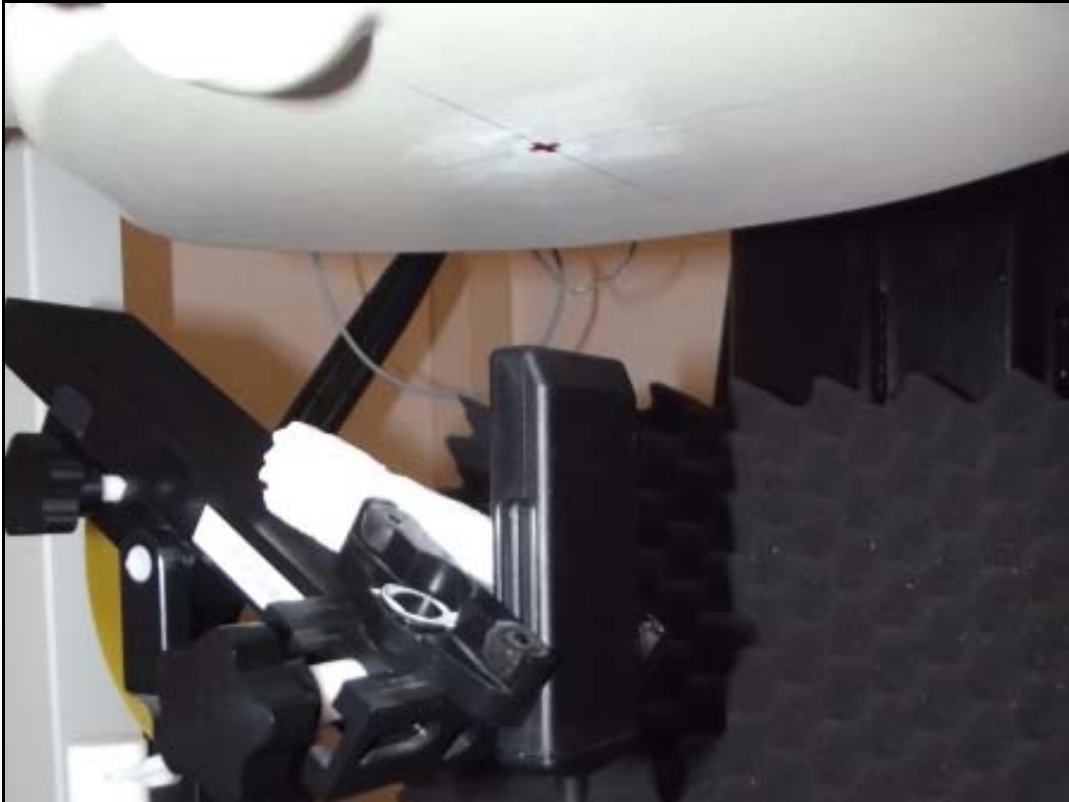
Photo 11: DUT - test position top edge with 5cm distance
