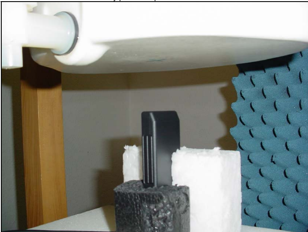
Photo 14: body position top side with 50mm distance
