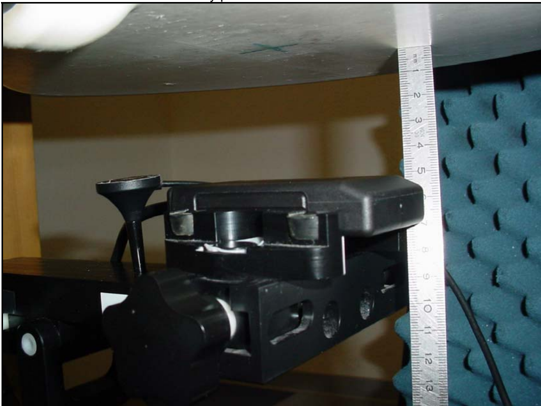
Photo 10: Test body position front side with 50mm distance
