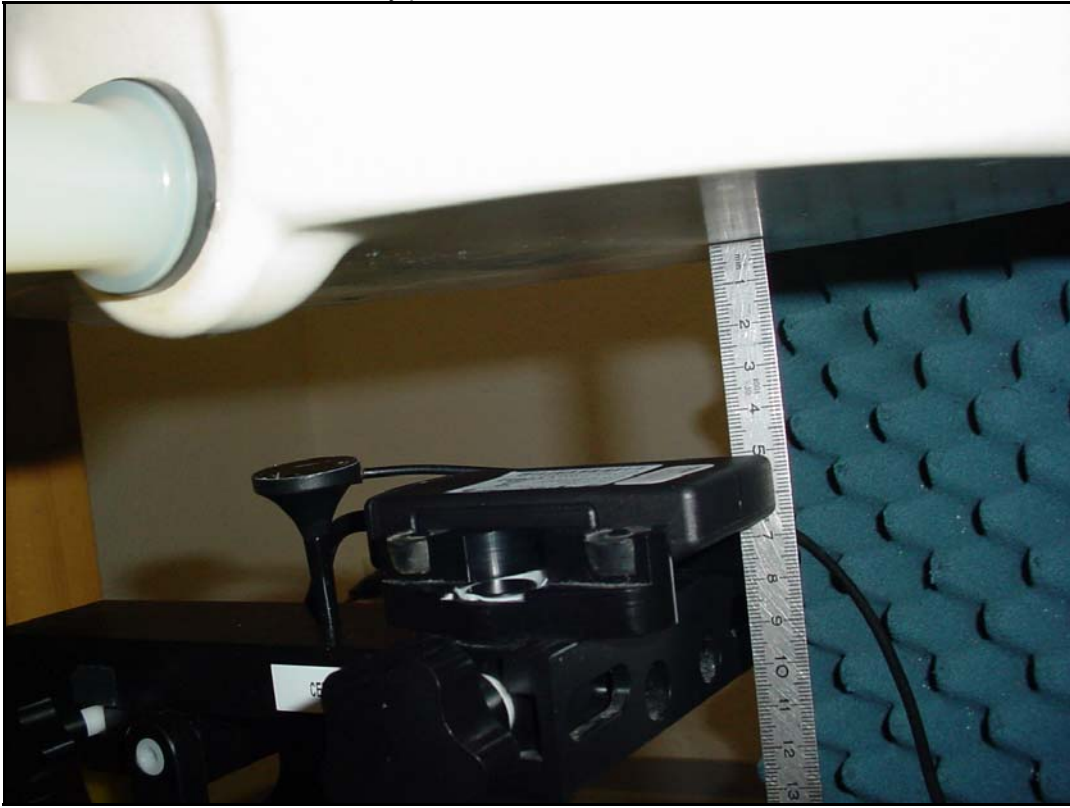
Photo 12: body position left side with 50mm distance
