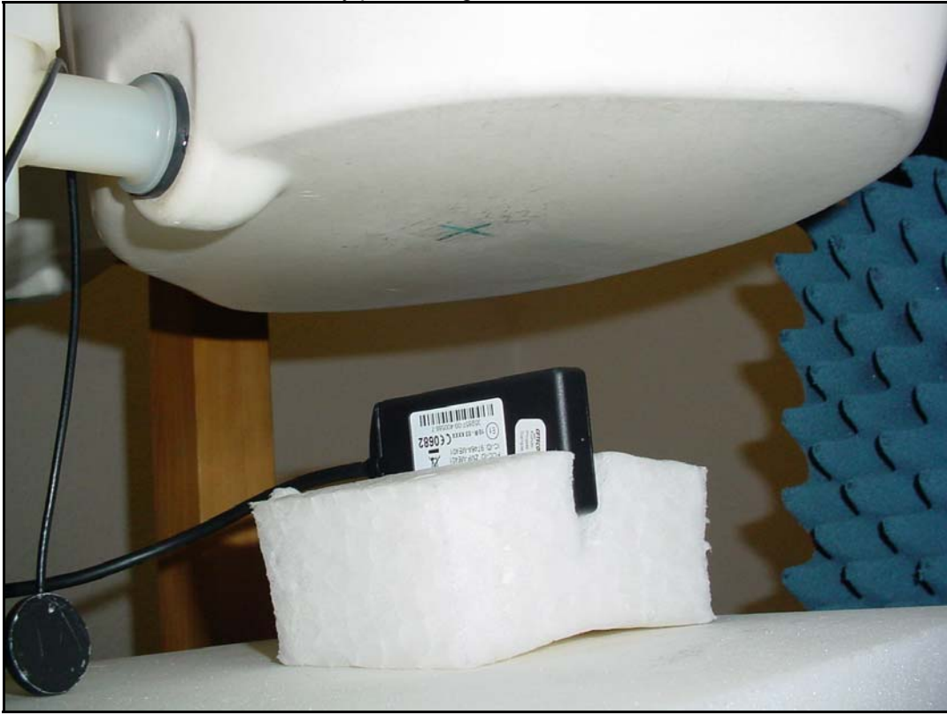
Photo 14: body position top side with 50mm distance
