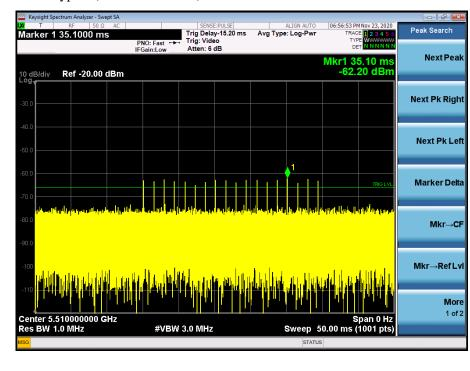
Radar Type 0 (40MHz / 5510Hz)
