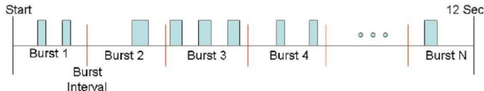
**Table D.7: Frequency Hopping Radar Test Waveform**
