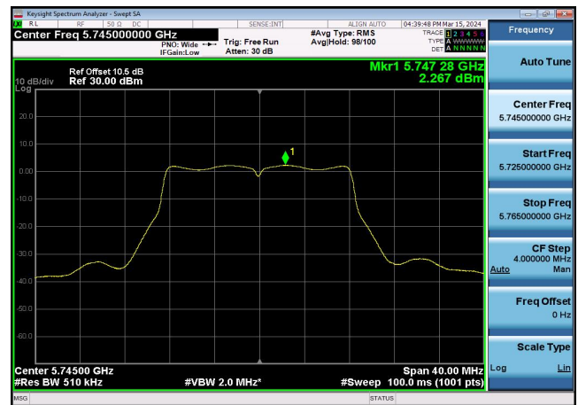
U-NII-3 Power spectral density-802.11 a(20MHz),5825MHz,Ant1
