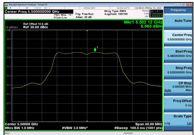
U-NII-2c Power spectral density-802.1 1a(20MHz),5700MHz,Ant1
