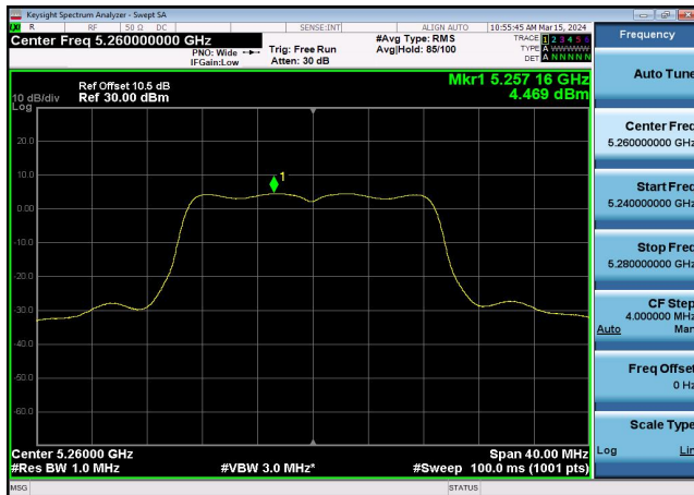
U-NII-2a Power spectral density-802.1 1n(20MHz),5320MHz,Ant1
