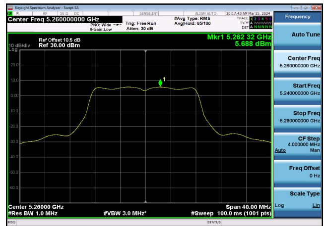
U-NII-2a Power spectral density-802.1 1a(20MHz),5320MHz,Ant1
