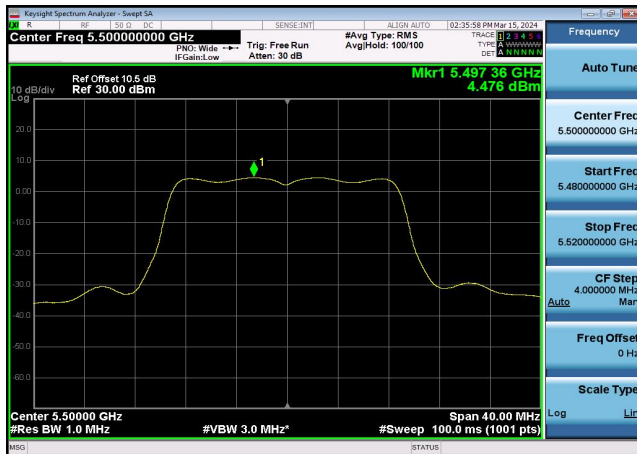
U-NII-2c Power spectral density-802.1 1n(20MHz),5700MHz,Ant1
