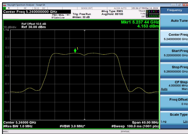
U-NII-1 Power spectral density-802.11 a(20MHz),5220MHz,Ant1
