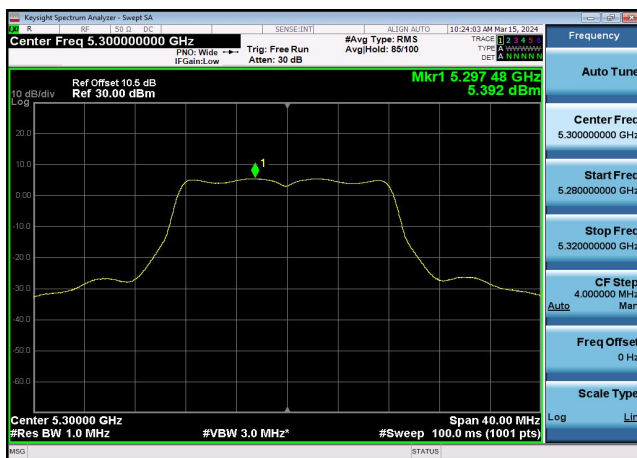
U-NII-2a Power spectral density-802.1 1a(20MHz),5300MHz,Ant1
