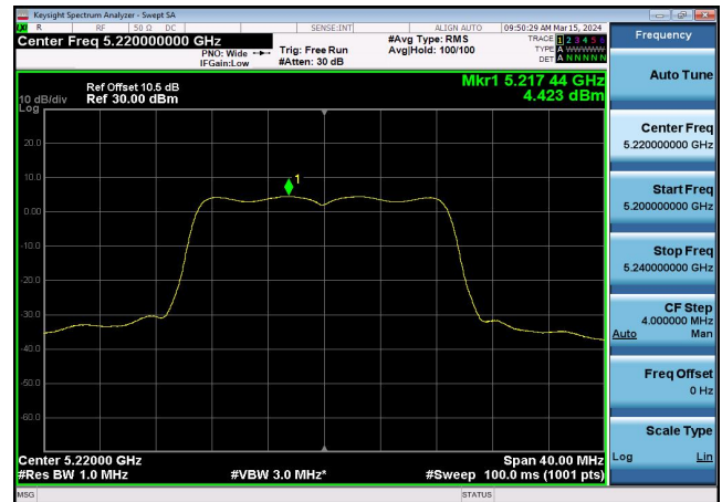
U-NII-1 Power spectral density-802.11 ax(20MHz),5180MHz,Ant1
