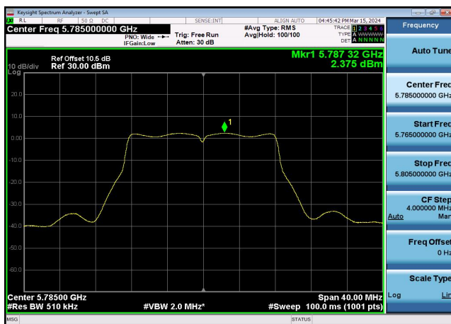
U-NII-3 Power spectral density-802.11 a(20MHz),5785MHz,Ant1
