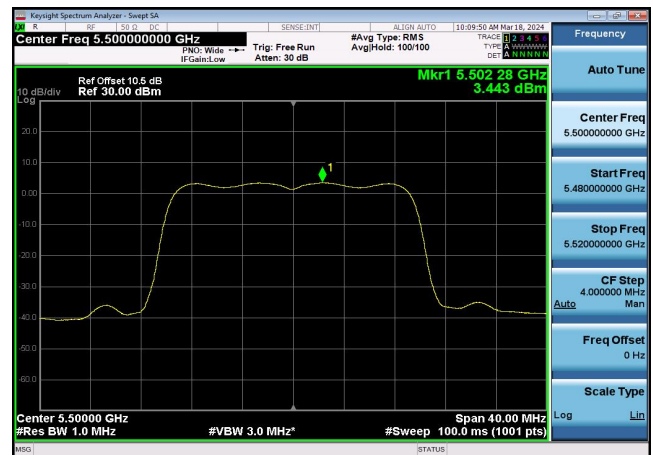
U-NII-2c Power spectral density-802.1 1ax(20MHz),5700MHz,Ant1
