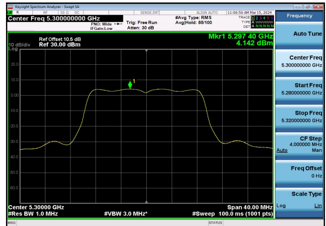
U-NII-2a Power spectral density-802.1 1ax(20MHz),5260MHz,Ant1
