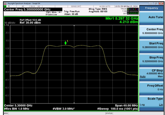
U-NII-2a Power spectral density-802.1 1a(20MHz),5260MHz,Ant1
