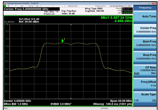
U-NII-2c Power spectral density-802.1 1ax(20MHz),5500MHz,Ant1
