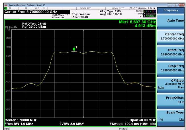
U-NII-2c Power spectral density-802.1 1a(20MHz),5700MHz,Ant1
