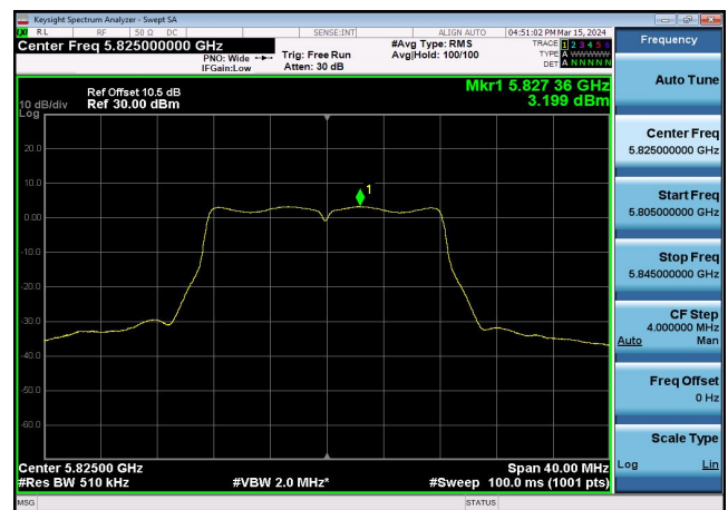
U-NII-3 Power spectral density-802.11 a(20MHz),5825MHz,Ant1
