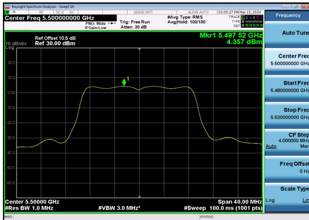
U-NII-2c Power spectral density-802.1 1ac(20MHz),5700MHz,Ant1
