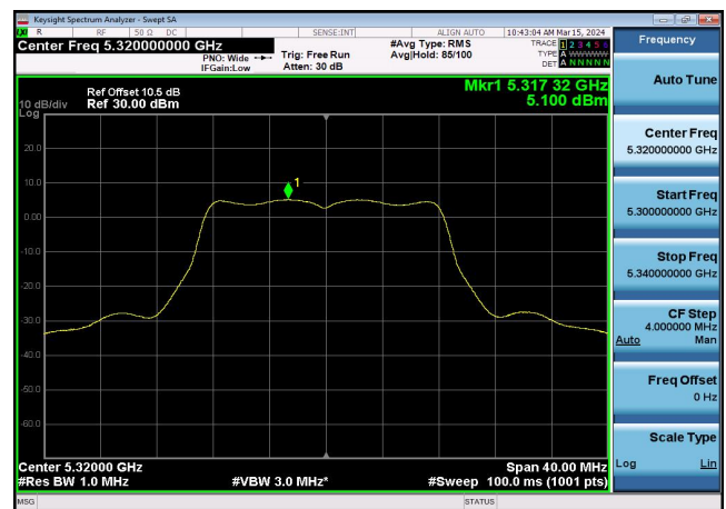
U-NII-2a Power spectral density-802.1 1a(20MHz),5320MHz,Ant1
