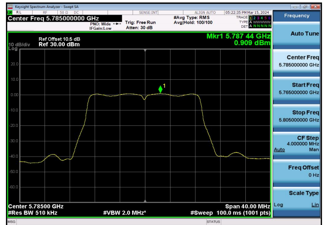
U-NII-3 Power spectral density-802.11 ax(20MHz),5745MHz,Ant1
