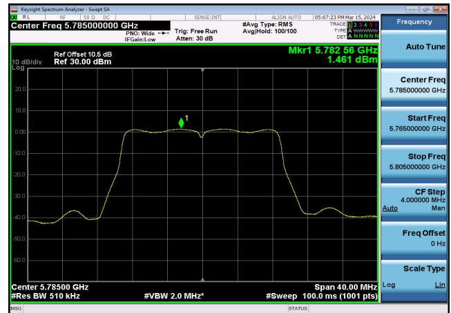
U-NII-3 Power spectral density-802.11 a(20MHz),5745MHz,Ant1
