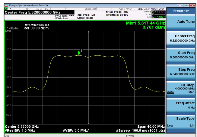
U-NII-2a Power spectral density-802.1 1ax(20MHz),5320MHz,Ant1
