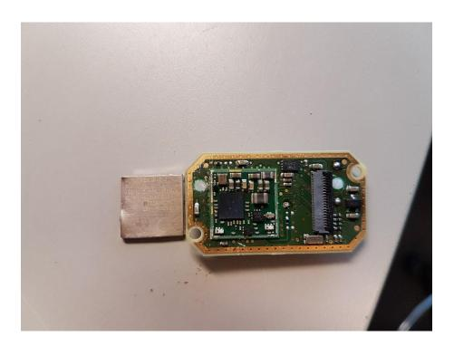
Figure 3 Radio module without cover.
