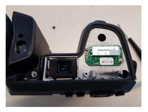
Figure 1 Radio board EVBW2 placed on top of LCD unit.
