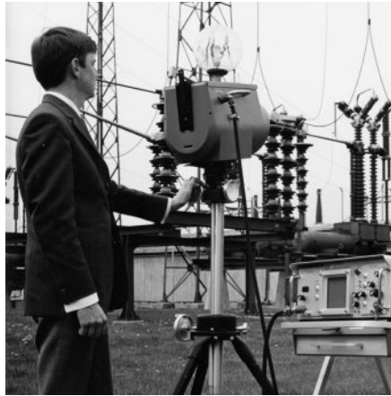
Figure 30.2 1969: Thermovision Model 661. The camera weighed approximately 25 kg (55 lb.), the oscilloscope 20 kg (44 lb.), and the tripod 15 kg (33 lb.). The operator also needed a 220 VAC generator set, and a 10 L (2.6 US gallon) jar with liquid nitrogen. To the left of the oscilloscope the Polaroid attachment (6 kg/13 lb.) can be seen.
