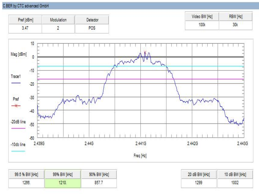
Plot 8: middle channel – 2441 MHz, 8 DPSK modulation
