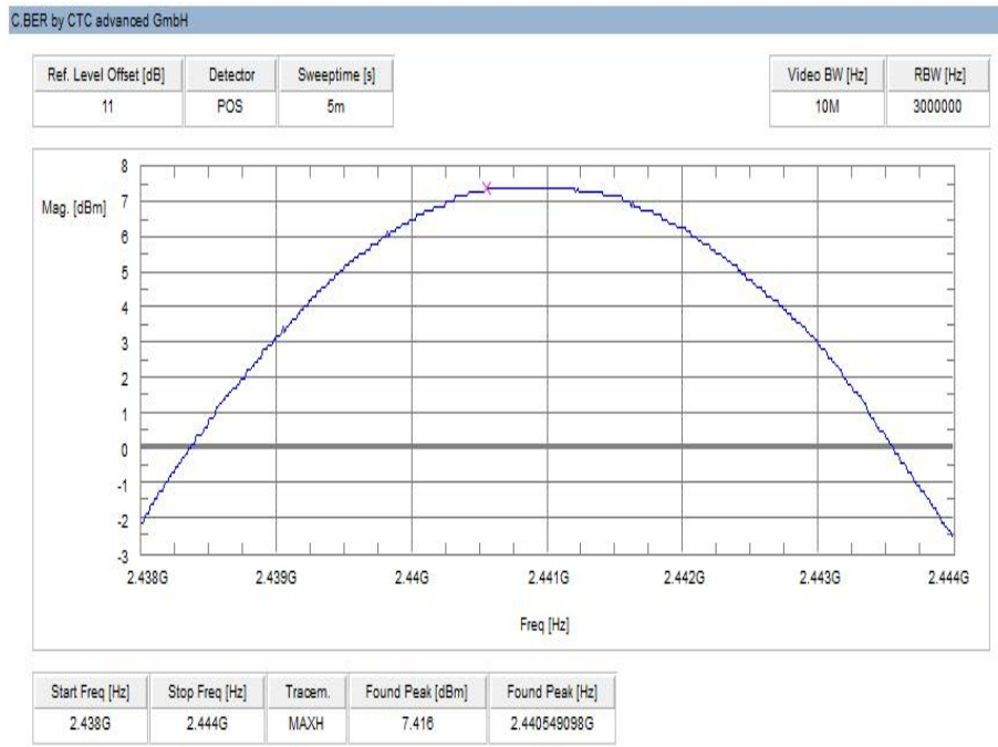
Plot 2: middle channel – 2441 MHz, GFSK modulation
