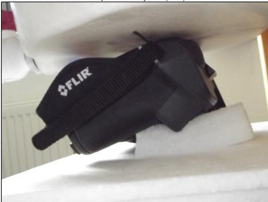
Photo 10: Measurement position – Body worn (Front) with 0mm distance
