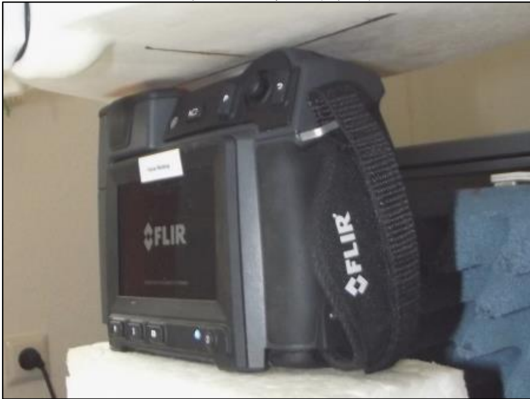
Photo 12: Measurement position – Body worn (Right side) with 0mm distance
