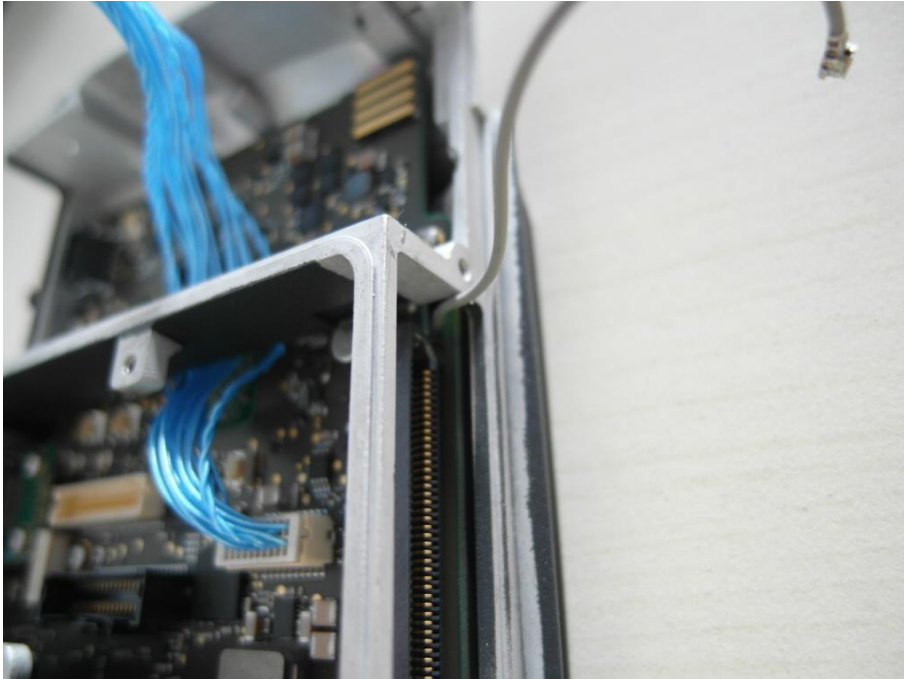
Photo 21: UFL RF cable through the housing
