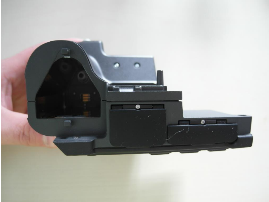
Photo 5: view on the battery compartment
