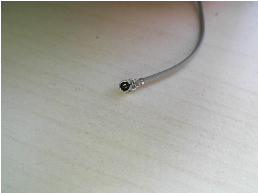
Photo 22: UFL connector at RF cable
