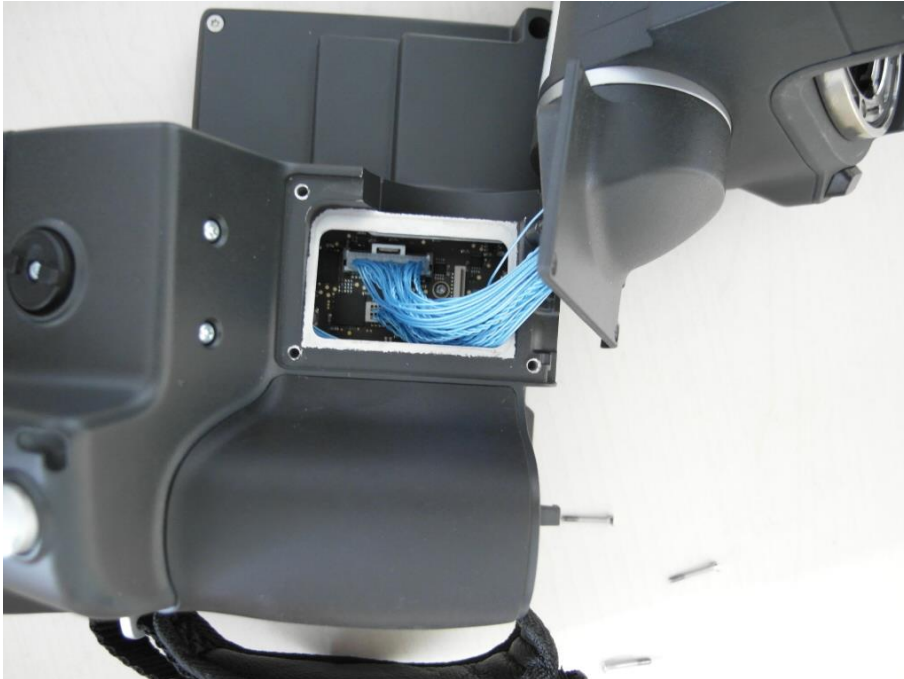
Photo 1: separation of main body and radiometric unit
