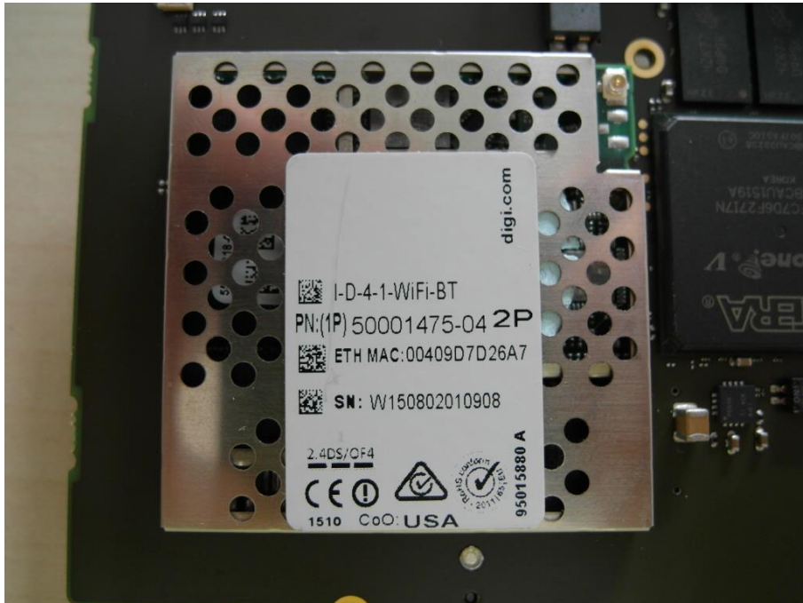
Photo 27: digi main module including RF part and UFL connector
