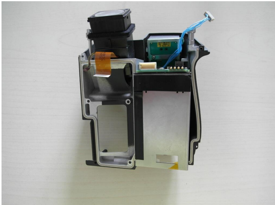
Photo 18: body part with battery connector board and view finder
