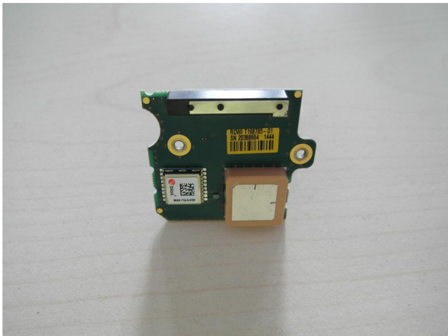
Photo 10: Antenna module with GPS chip
