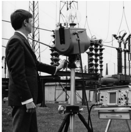
Figure 28.2 1969: Thermovision Model 661. The camera weighed approximately 25 kg (55 lb.), the oscilloscope 20 kg (44 lb.), and the tripod 15 kg (33 lb.). The operator also needed a 220 VAC generator set, and a 10 L (2.6 US gallon) jar with liquid nitrogen. To the left of the oscilloscope the Polaroid attachment (6 kg/13 lb.) can be seen.
