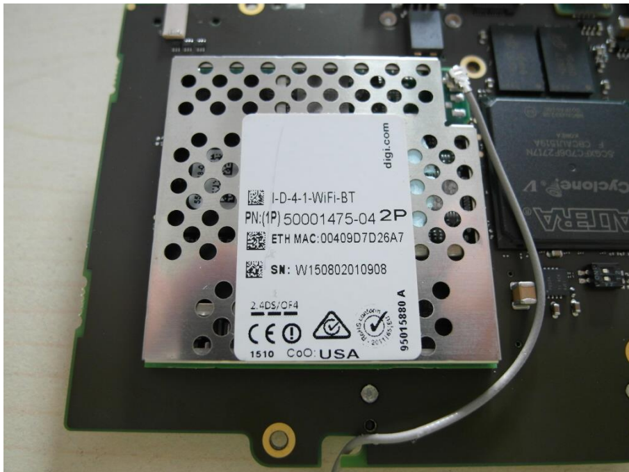
Photo 26: digi main module including RF part and RF cable
