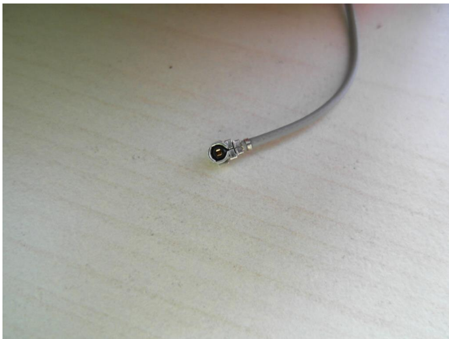
Photo 22: UFL connector at RF cable
