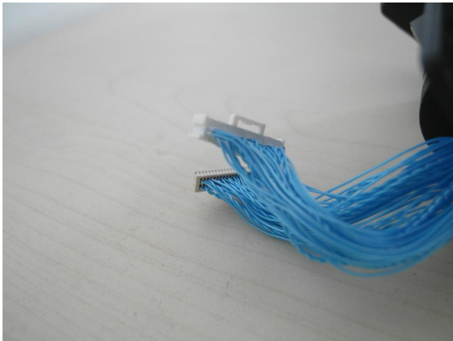
Photo 3: connection cables between main pc board and radiometric unit
