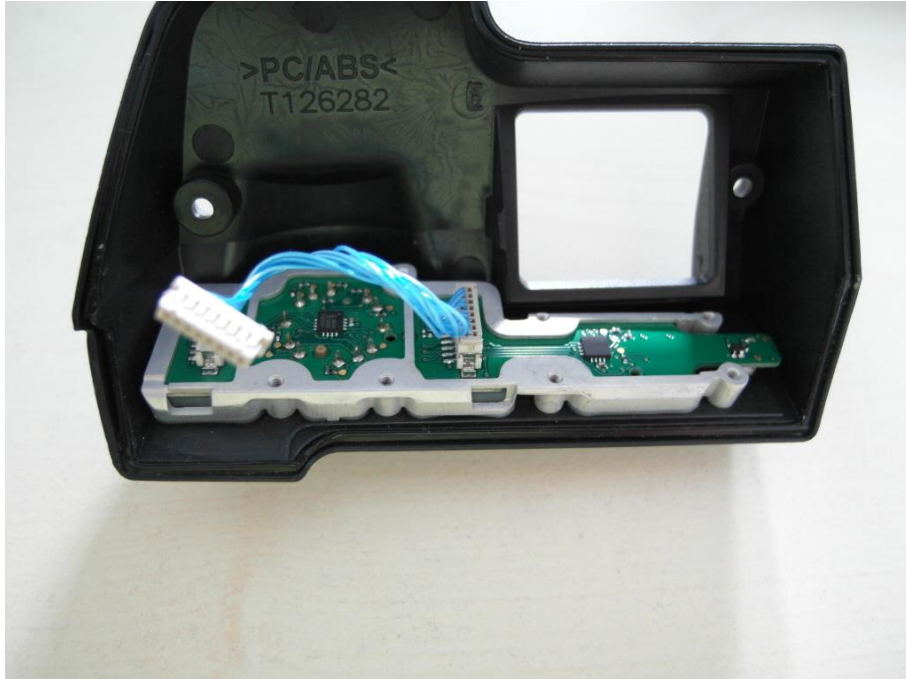
Photo 7: Top of the camera with the PCB for the buttons and joystick
