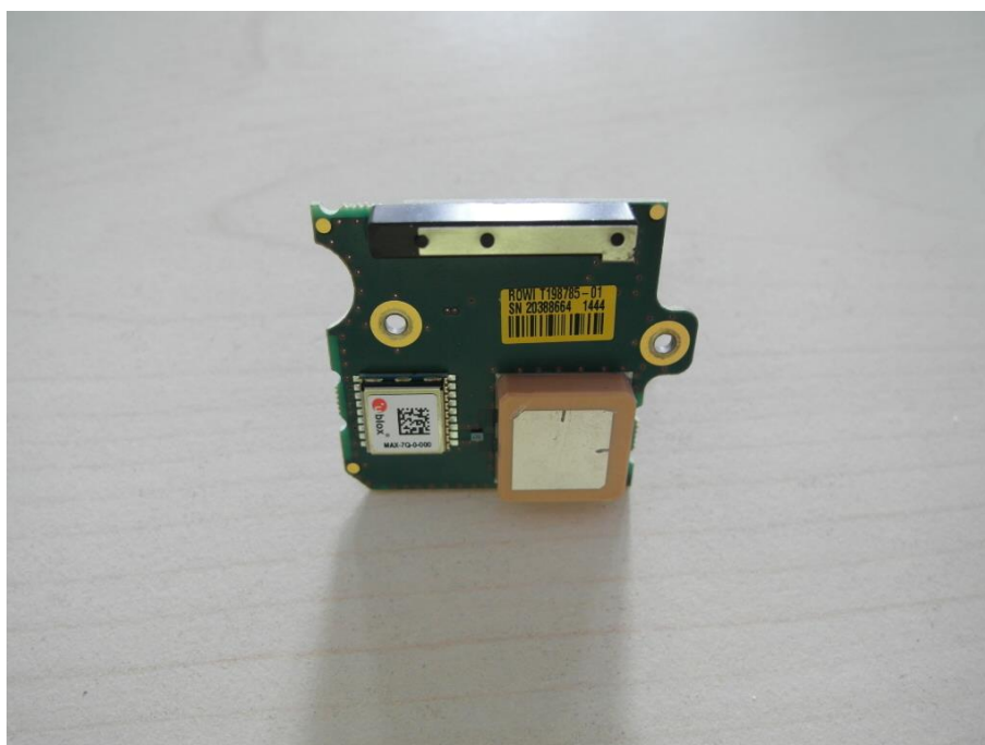
Photo 10: Antenna module with GPS chip
