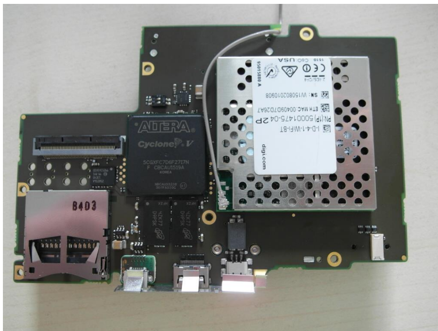
Photo 29: Main PC board with antenna cable for BT/WLAN
