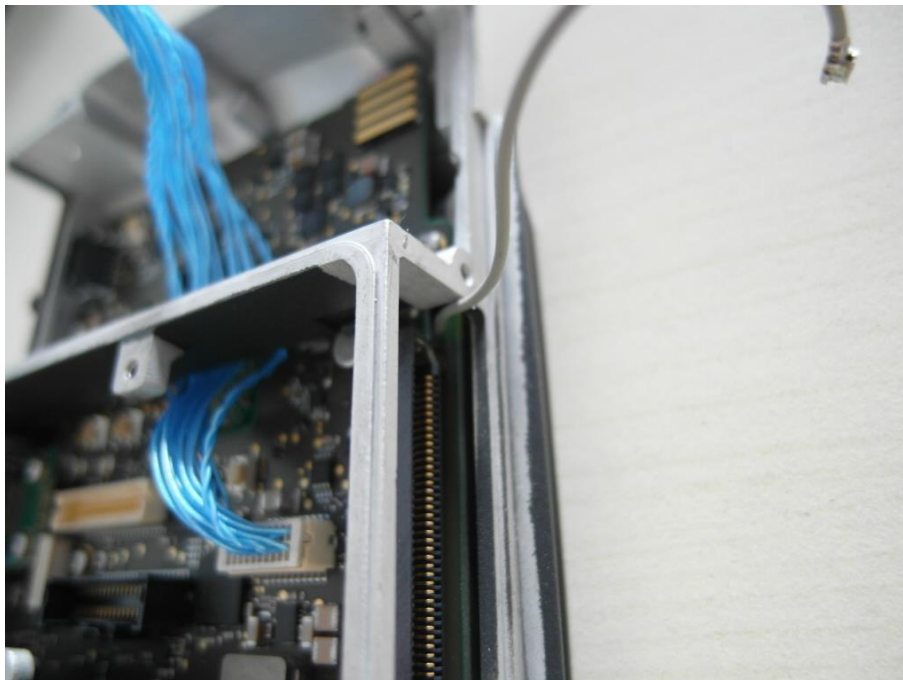
Photo 21: UFL RF cable thru the housing
