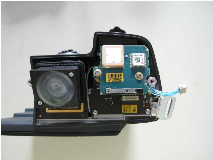
Photo 8: Top view – GPS antenna, GPS module and BT/WLAN antenna
