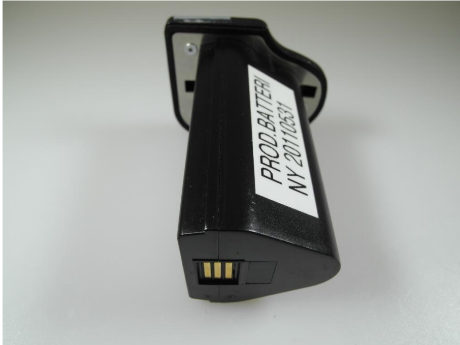
Photo 11: battery interface port
