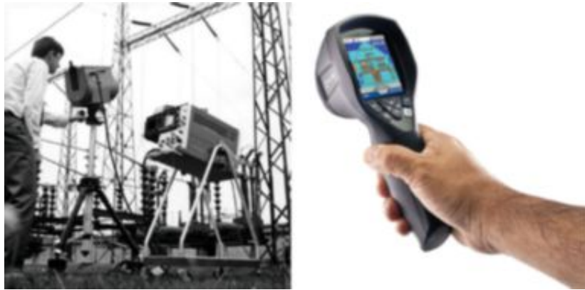
Figure 28.2 LEFT: Thermovision Model 661 from 1969. The camera weighed approximately 25 kg (55 lb.), the oscilloscope 20 kg (44 lb.), and the tripod 15 kg (33 lb.). The operator also needed a 220 VAC generator set, and a 10 L (2.6 US gallon) jar with liquid nitrogen. To the left of the oscilloscope the Polaroid attachment (6 kg/13 lb.) can be seen. RIGHT: Flir i7 from 2012. Weight: 0.34 kg (0.75 lb.), including the battery.
