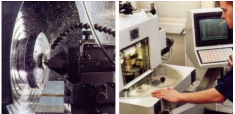
Figure 28.4 LEFT: Diamond turning machine; RIGHT: Lens polishing
