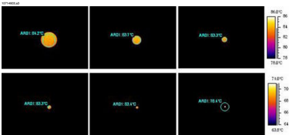
Figure 29.20 Temperature readings from a blackbody at +85°C (+185°F) at increasing distances (24° lens)
