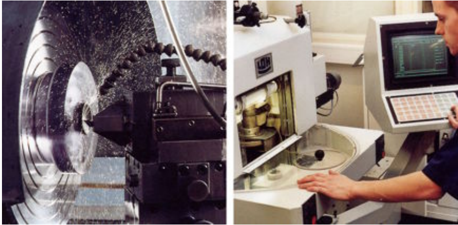
Figure 30.4 LEFT: Diamond turning machine; RIGHT: Lens polishing
