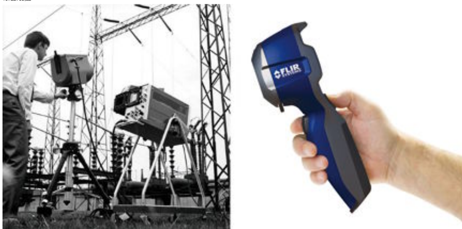
Figure 30.2 LEFT: Thermovision® Model 661 from 1969. The camera weighed approximately 25 kg (55 lb.), the oscilloscope 20 kg (44 lb.), and the tripod 15 kg (33 lb.). The operator also needed a 220 VAC generator set, and a 10 L (2.6 US gallon) jar with liquid nitrogen. To the left of the oscilloscope the Polaroid attachment (6 kg/13 lb.) can be seen. RIGHT: FLIR i7 from 2009. Weight: 0.34 kg (0.75 lb.), including the battery.
