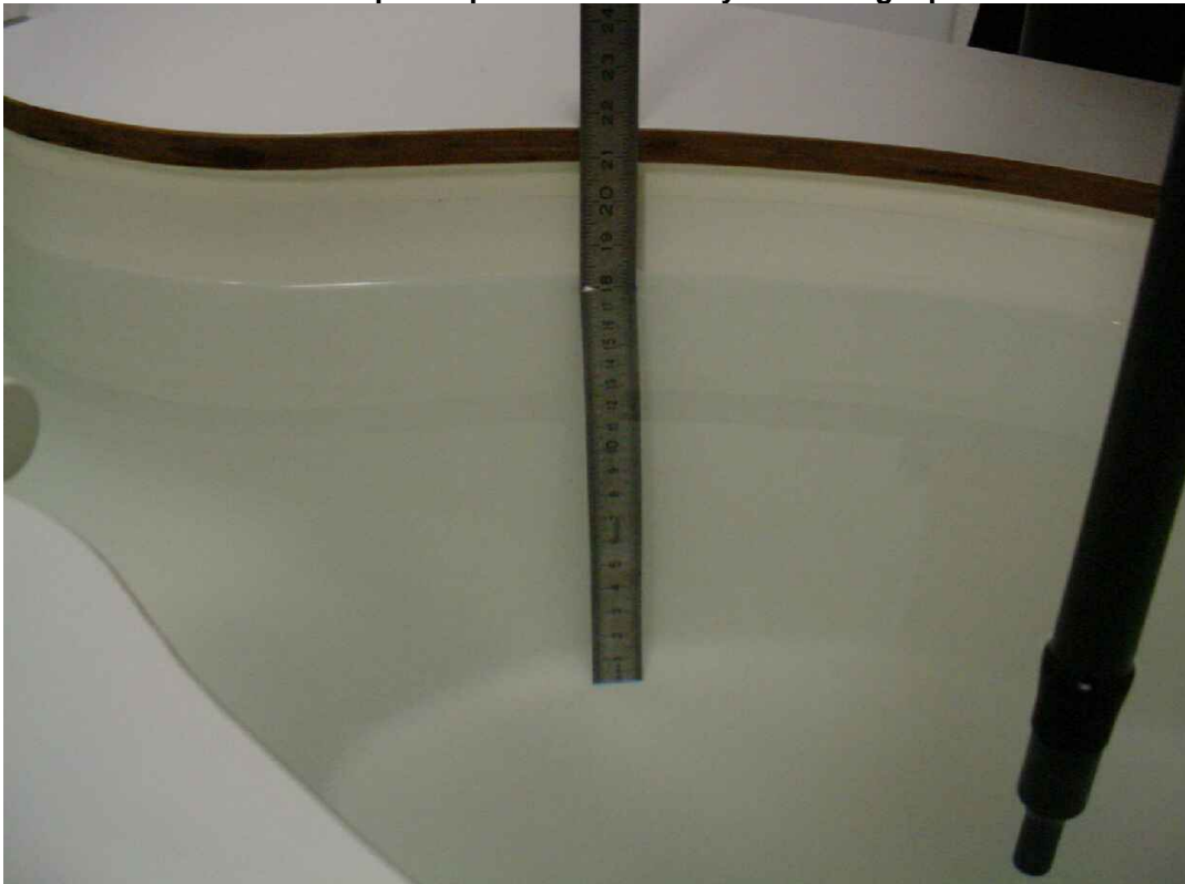
Photo 2: Liquid depth 2450 MHz body simulating liquid
