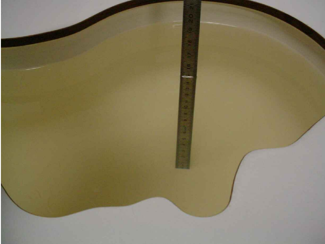
Photo 2: Liquid depth 2450 MHz body simulating liquid
