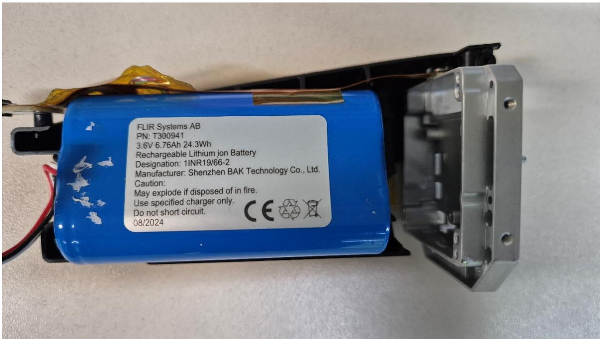
Figure 12 FLIR-O1500, Battery Pack T300941.
