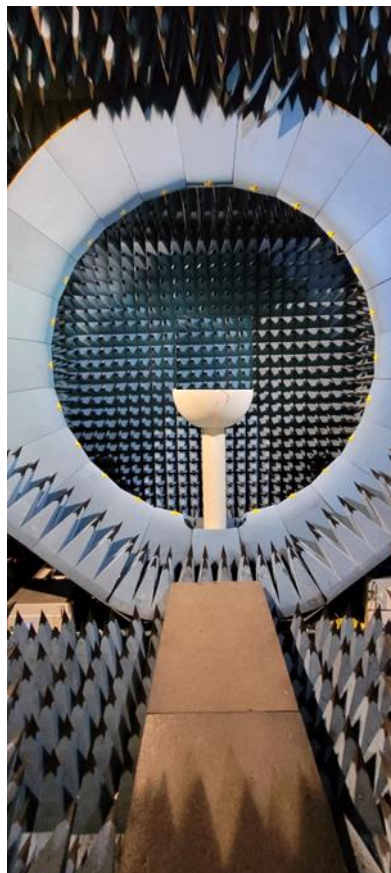
Figure 5-4 Satimo SG-23 6 GHz Stargate Antenna Test Chamber
