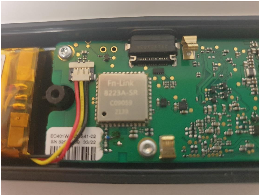
Figure 6 Radio Module, Fn-Link 8223A-SR, in the FLIR ONE Edge.
