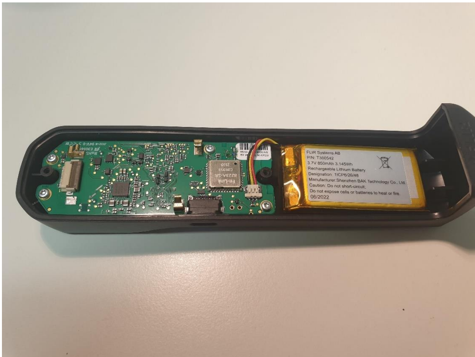
Figure 4 Inside of the FLIR ONE Edge, Back panel removed.
