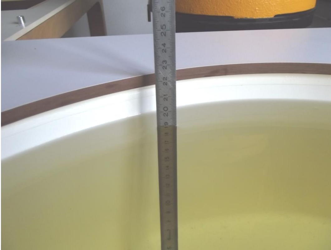
Photo 2: Liquid depth 5 GHz body simulating liquid
