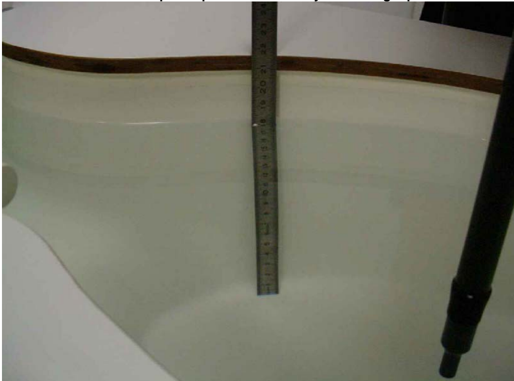
Photo 1: Liquid depth 2450 MHz body simulating liquid
