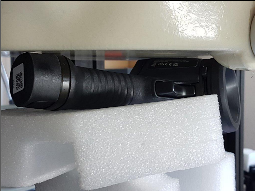
Photo 13: Test position - right side with 0mm distance
