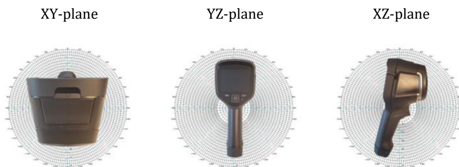
Figure 5-3 Measurement plane definition
