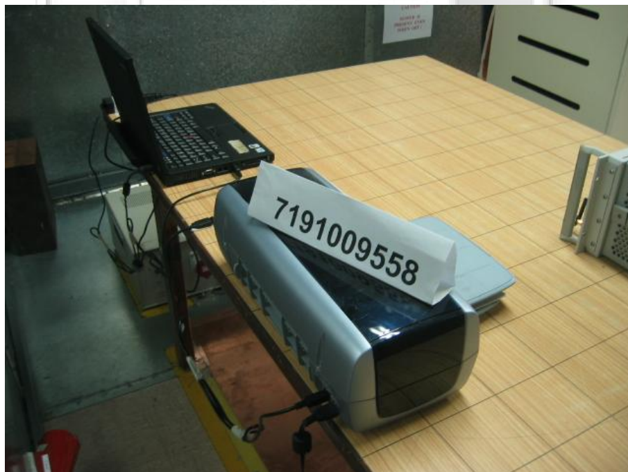
Conducted Emissions Test Setup (Rear View)
