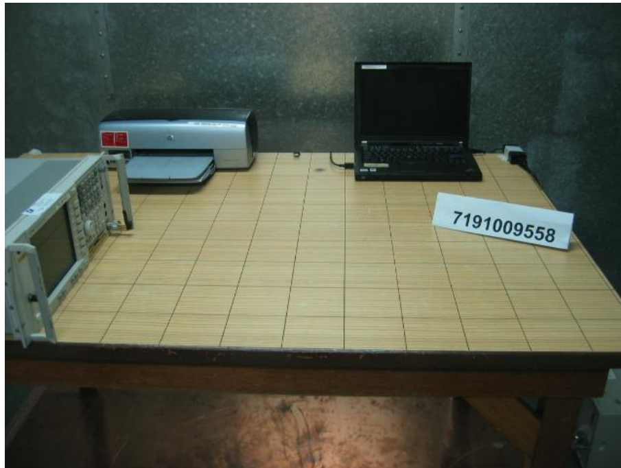
Conducted Emissions Test Setup (Front View)
