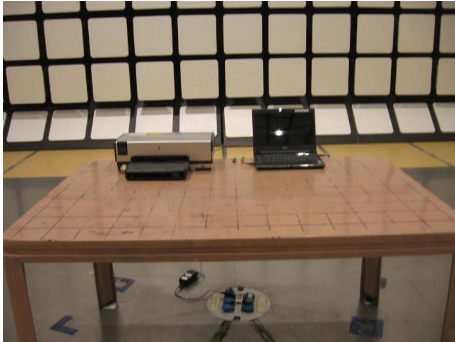
Radiated Emissions Test Setup (Front View)
