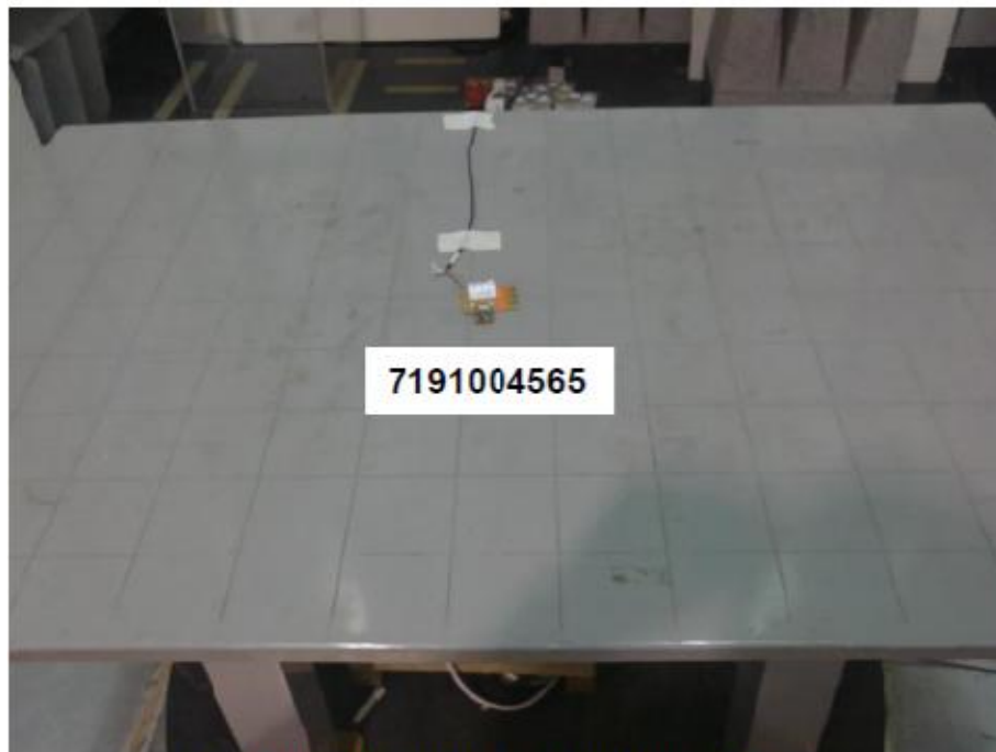
Radiated Emissions Test Setup (Front View)
