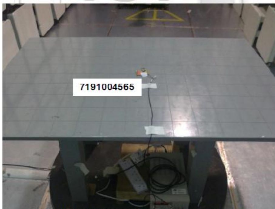
Radiated Emissions Test Setup (Rear View)
