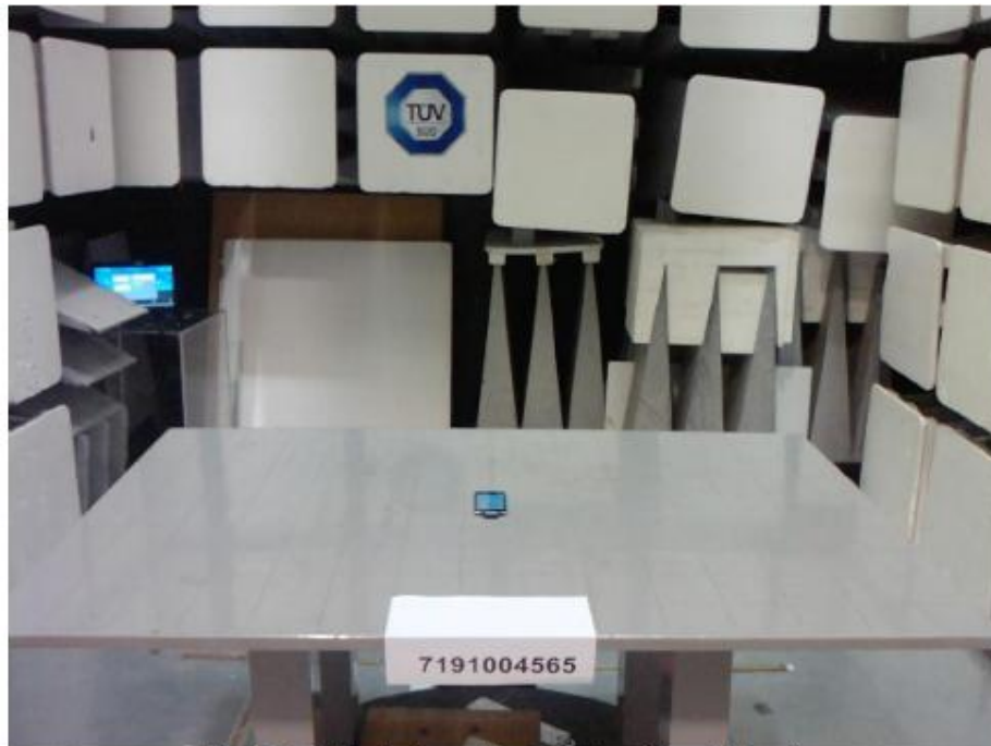
Radiated Emissions Test Setup (Front View)
