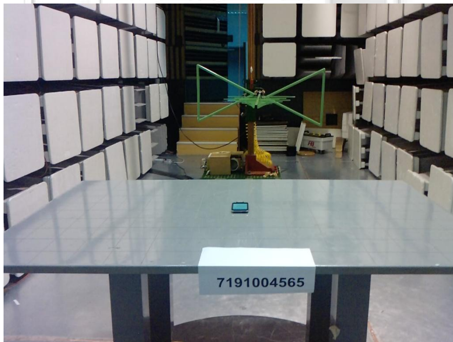
Radiated Emissions Test Setup (Rear View)
