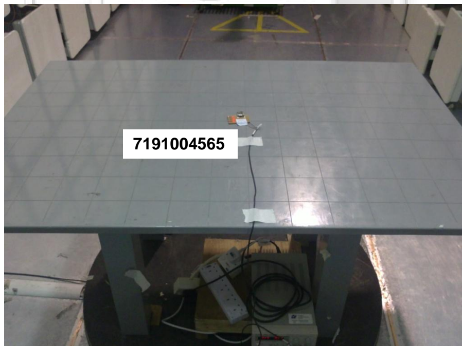
Radiated Emissions Test Setup (Rear View)
