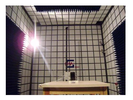
Radiation Spurious Emission Test Setup (Above 1GHz)
