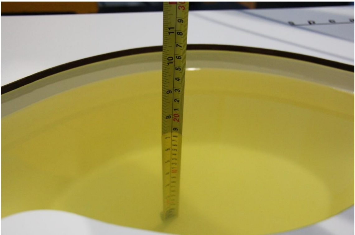
Picture 7-12: Liquid depth in the Flat Phantom(2550MHz)
