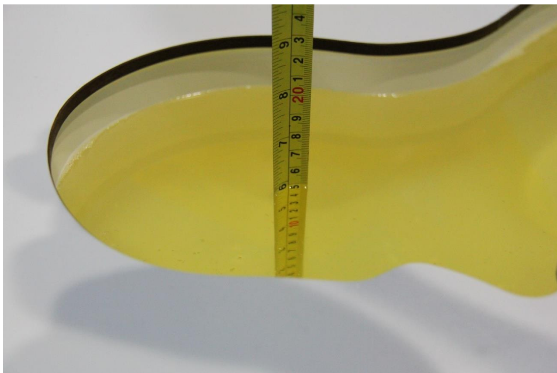
Picture 7-9: Liquid depth in the Head Phantom(2450MHz)
