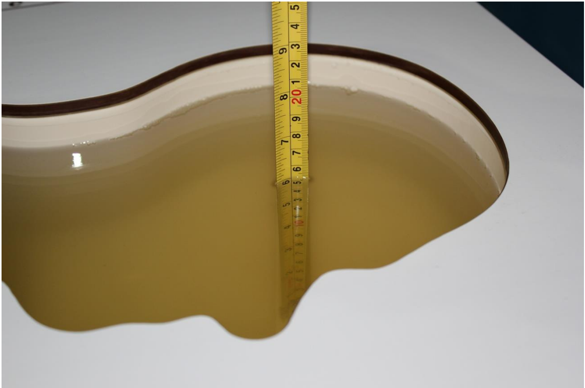
Picture 7-11: Liquid depth in the Head Phantom(2550MHz)
