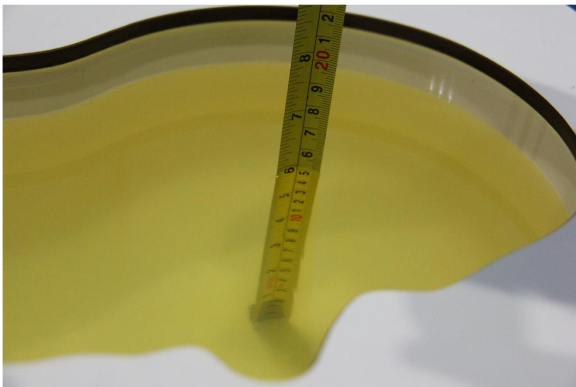
Picture 7-5: Liquid depth in the Head Phantom (1800 MHz)
