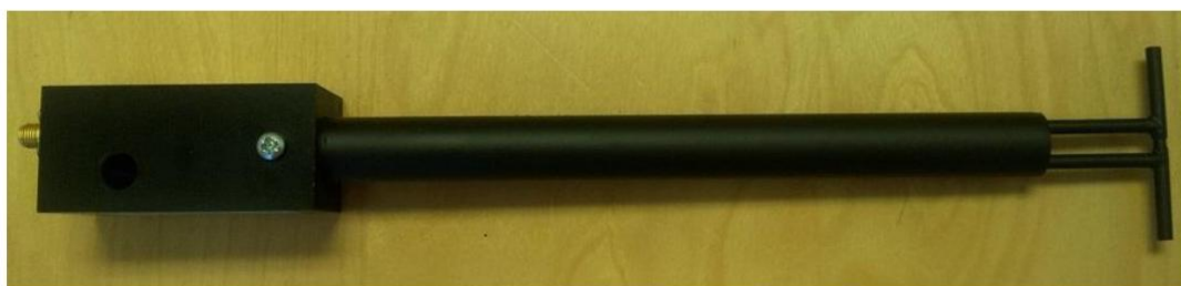
Figure 1 – MVG COMOSAR Validation Dipole
