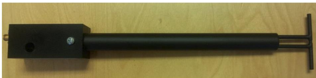
Figure 1 – MVG COMOSAR Validation Dipole
