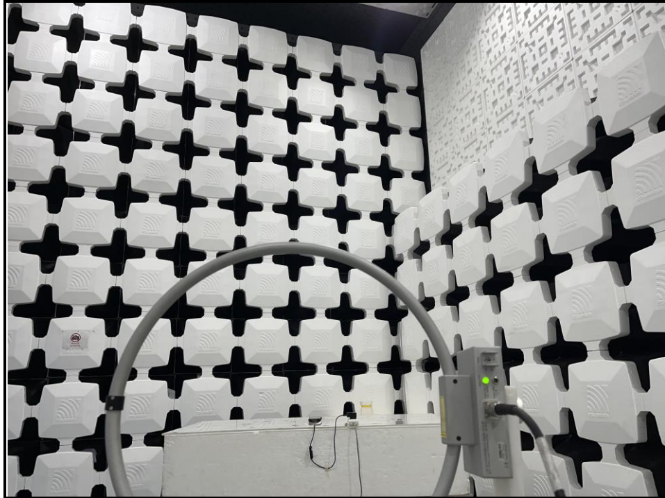
Fig. 1 Radiated emission setup photo(Below 30MHz)
