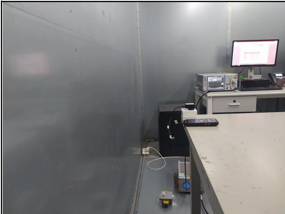
Fig. 4 Power line conducted emission setup photo
