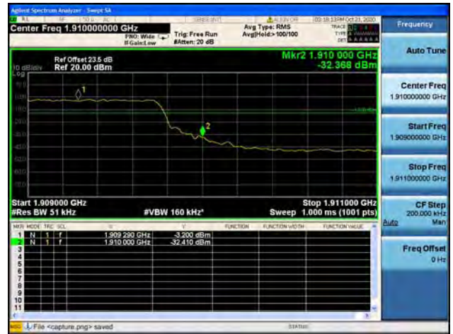
Band2 / 5MHz / High CH / 16QAM / FULL RB
