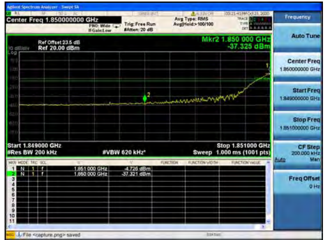
Band2 / 20MHz / Low CH / 16QAM / FULL RB
