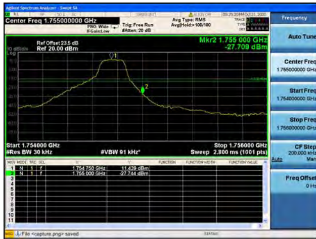
Band4 / 3MHz / High CH / 16QAM / 1 RB
