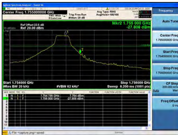
Band4 / 1.4MHz / High CH / 16QAM / 1 RB
