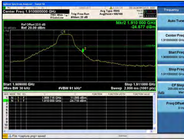
Band2 / 3MHz / High CH / 16QAM / 1 RB
