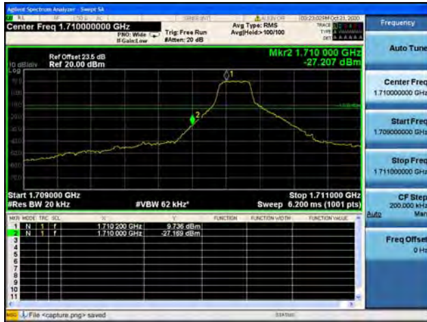
Band4 / 1.4MHz / Low CH / 16QAM / 1 RB
