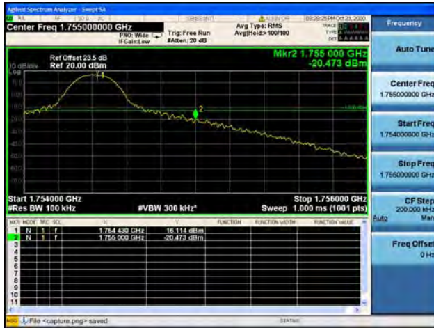
Band4 / 10MHz / High CH / 16QAM / 1 RB
