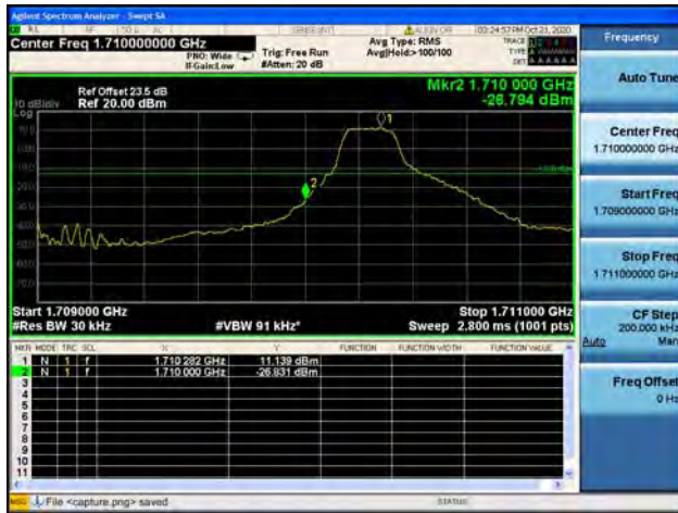
Band4 / 3MHz / Low CH / 16QAM / 1 RB
