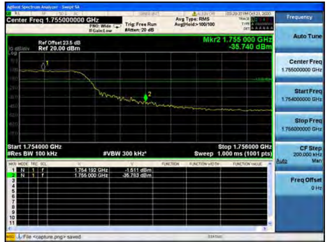
Band4 / 10MHz / High CH / 16QAM / FULL RB
