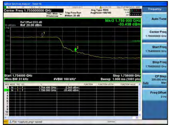
Band4 / 5MHz / High CH / 16QAM / FULL RB
