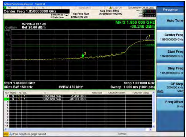
Band2 / 15MHz / Low CH / 16QAM / FULL RB
