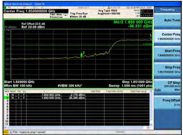
Band2 / 10MHz / Low CH / 16QAM / FULL RB
