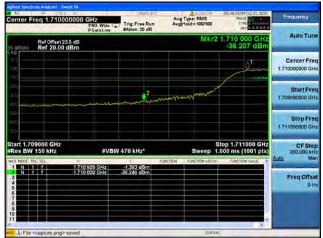
Band4 / 15MHz / Low CH / 16QAM / FULL RB
