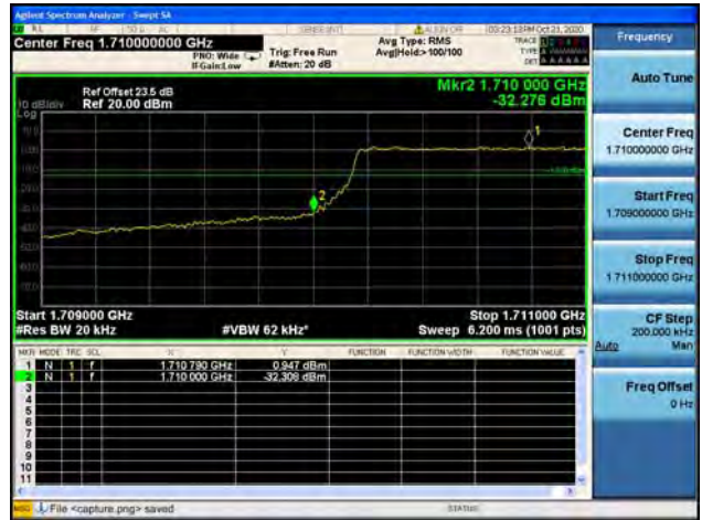
Band4 / 1.4MHz / Low CH / 16QAM / FULL RB
