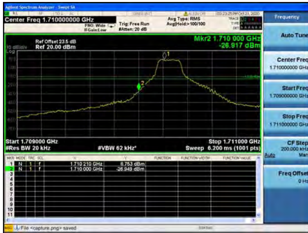
Band4 / 1.4MHz / Low CH / 16QAM / 1 RB
