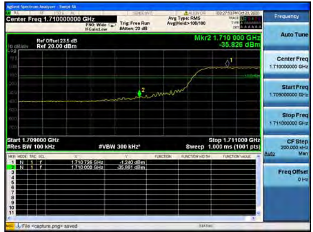
Band4 / 10MHz / Low CH / 16QAM / FULL RB
