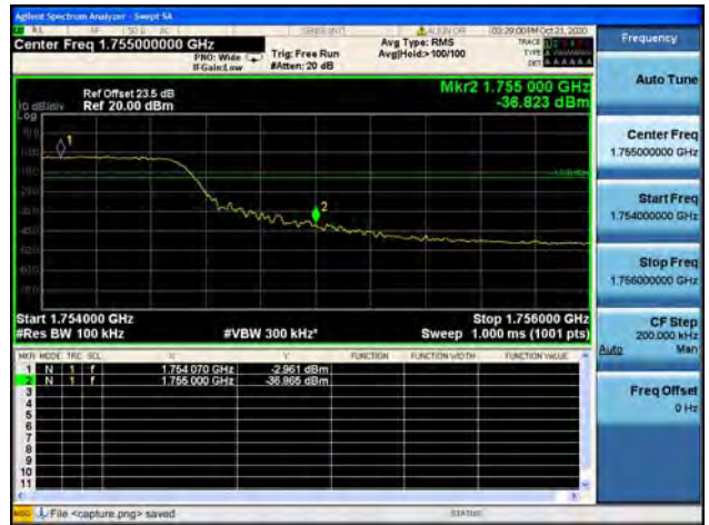
Band4 / 10MHz / High CH / 16QAM / FULL RB
