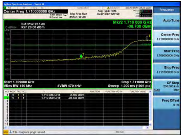
Band4 / 15MHz / Low CH / 16QAM / FULL RB
