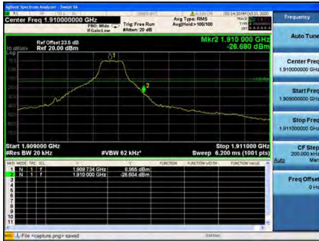
Band2 / 1.4MHz / High CH / 16QAM / 1 RB
