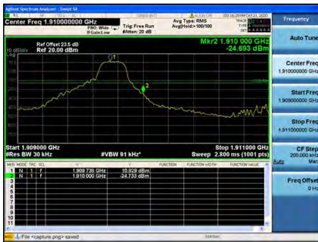
Band2 / 3MHz / High CH / 16QAM / 1 RB
