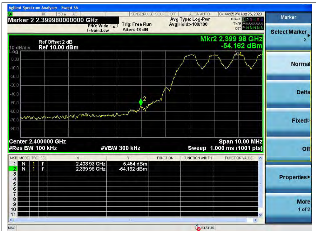
(Band edge with hopping on, Channel 0, GFSK)
