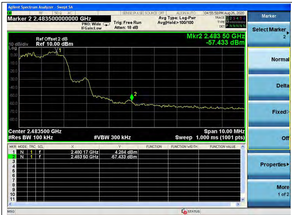
(Band edge with hopping on, Channel 78, 8-DPSK)
