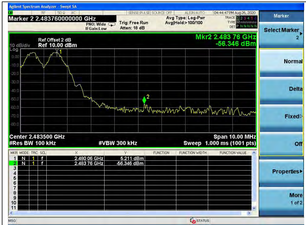
(Band edge with hopping on, Channel 78, GFSK)
