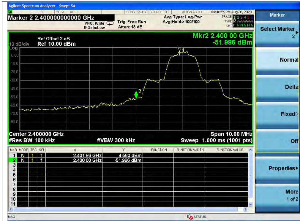
(Band edge, Channel 0, \pi/4 -DQPSK)
