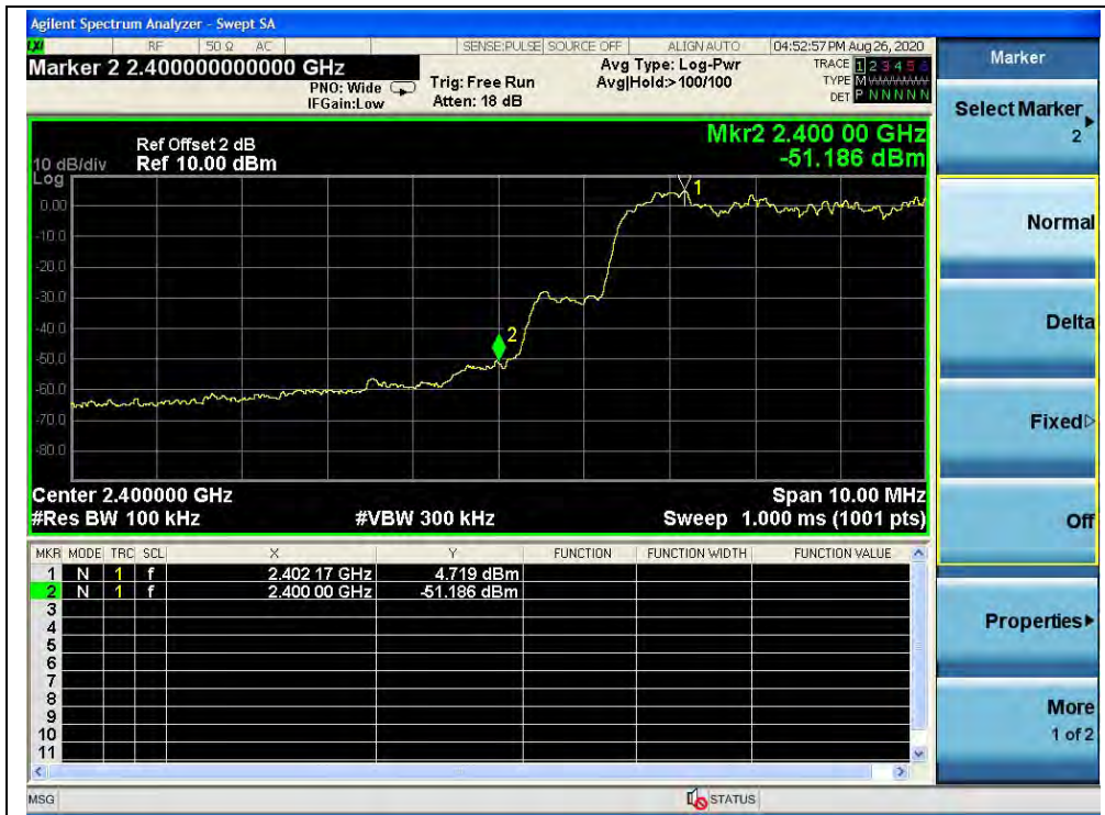
(Band edge with hopping on, Channel 0, 8-DPSK)
