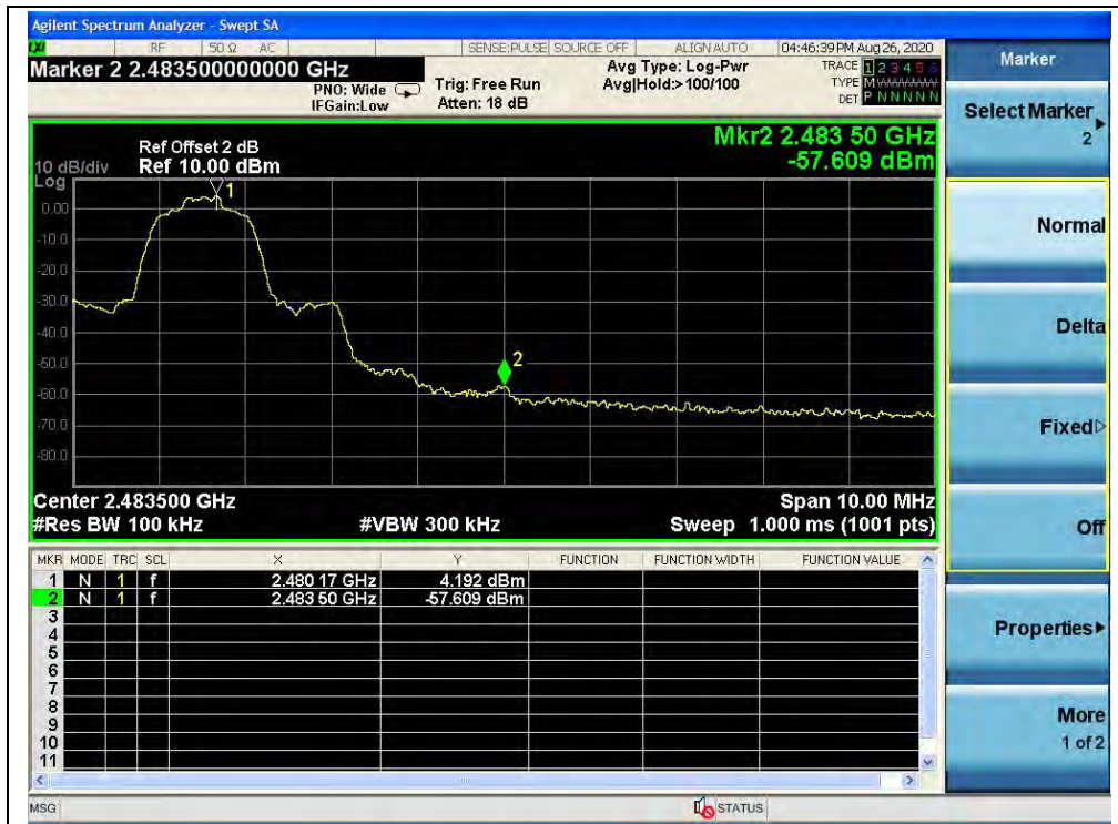
(Band edge, Channel 78, \pi/4 -DQPSK)
