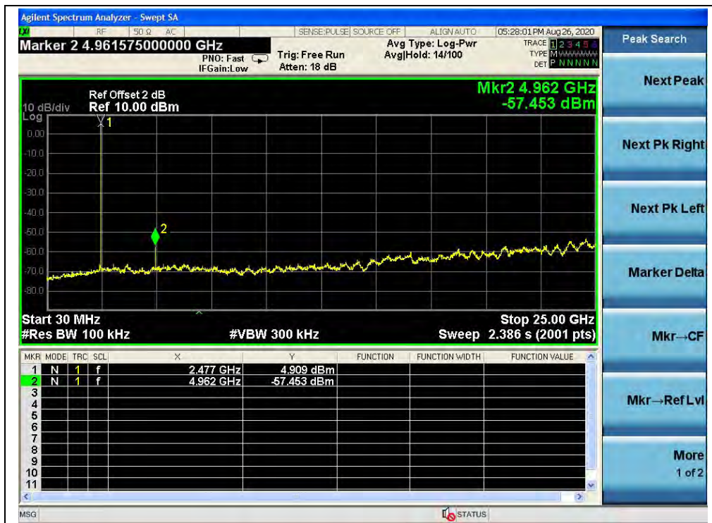
(30MHz to 25GHz, Channel 78, GFSK)
