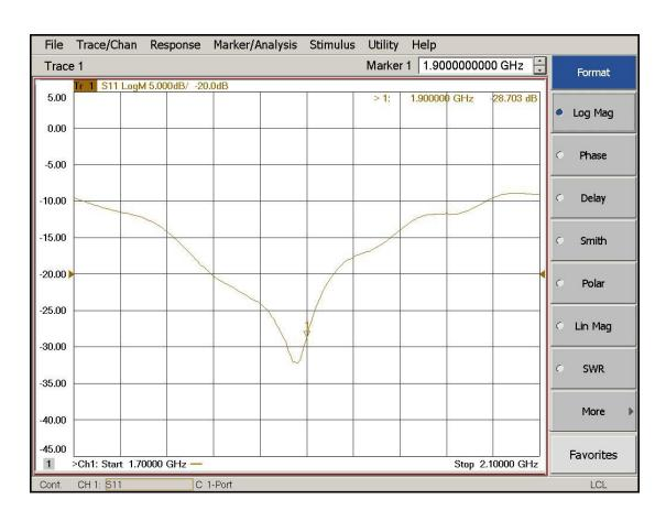
Impedance and Return Loss Test-Body(2016.2.19)
