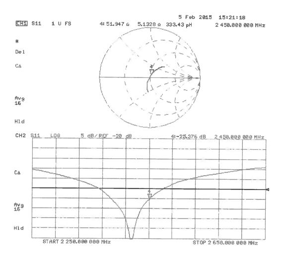
Impedance and Return Loss Test-Head(2016.2.19)
