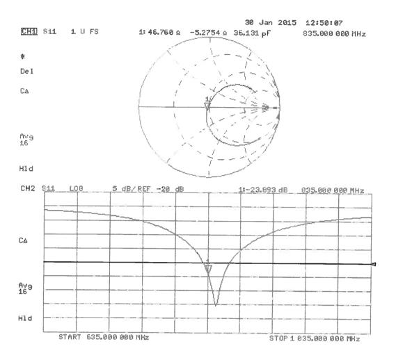
Impedance and Return Loss Test-Head(2016.2.19)
