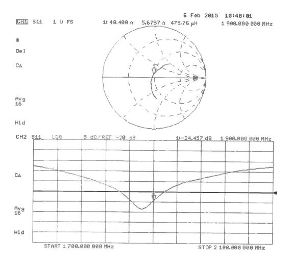
Impedance and Return Loss Test-Head(2016.2.19)
