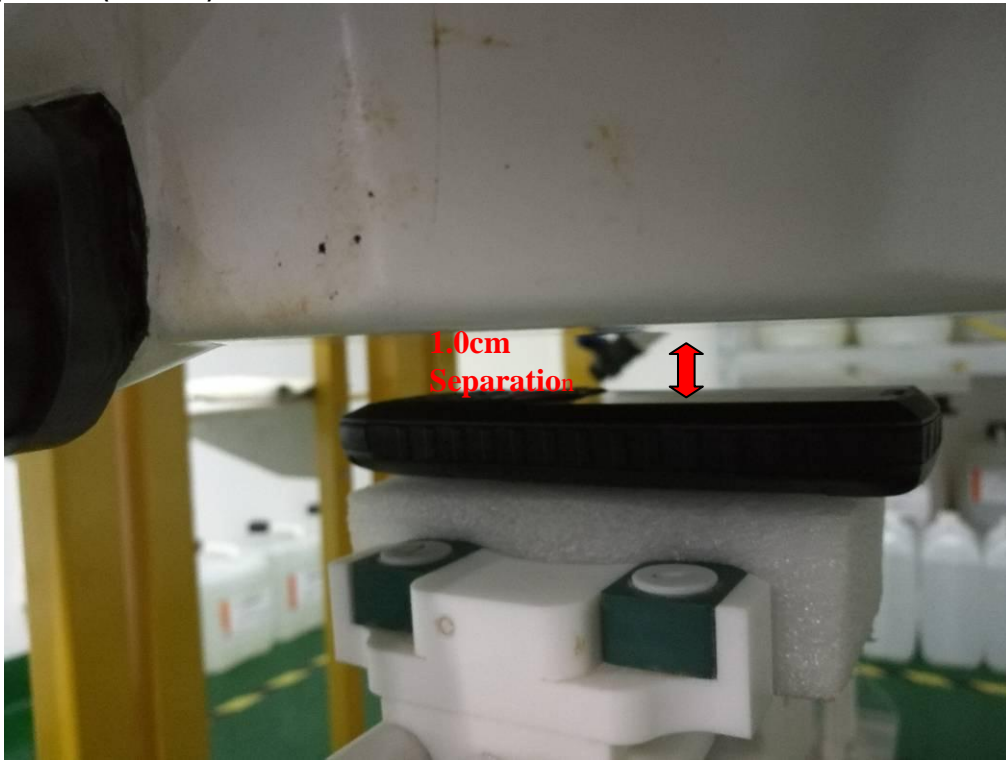
Body Setup Photo (LCD DOWN)
