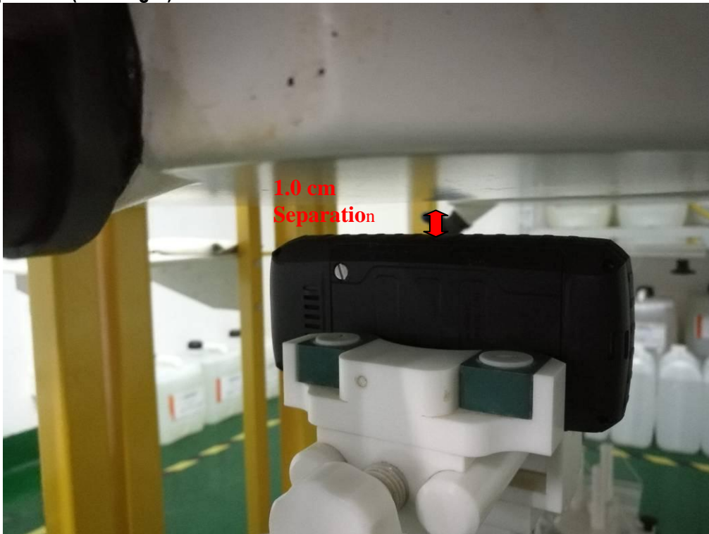
Body Setup Photo (LCD Right)
