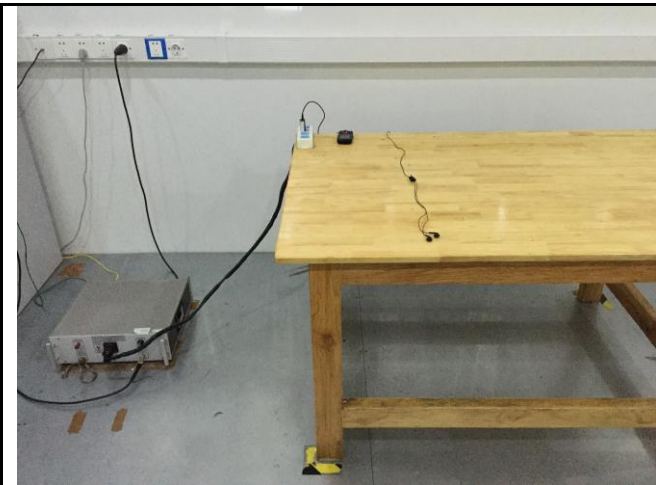
Conducted Emissions Test Setup Front View
